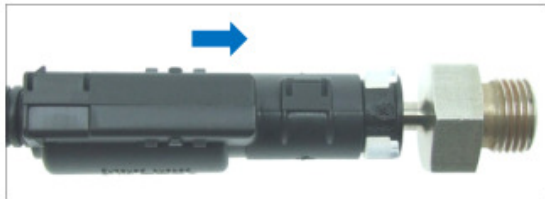
Fig. 5: Pushing the coupling as far as it will go onto the male connector; in the process the holding clip engages
