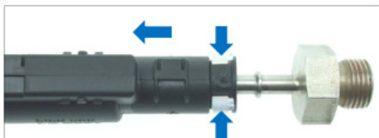
Fig. 8: Compressing the lugs of the holding clip and pulling the coupling off
