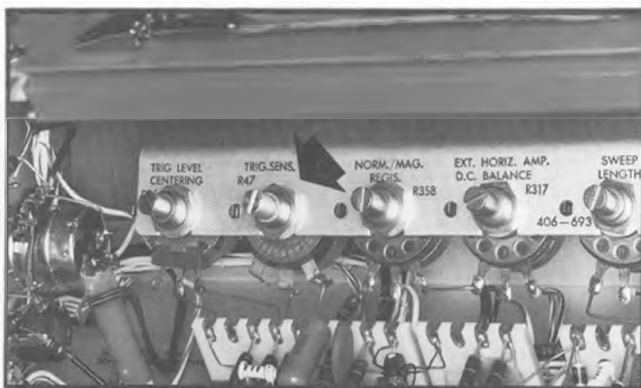
Fig. 2-9. TRIG. SENS. control location.
