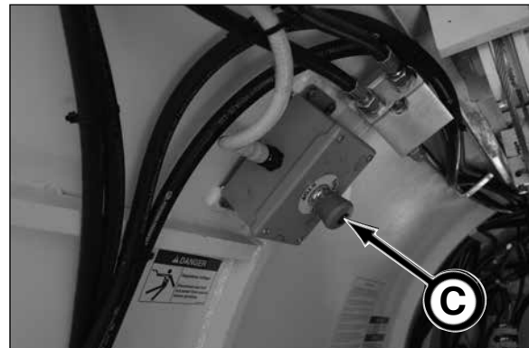
E-Stop on Series II TBM
