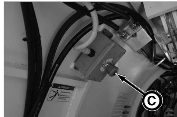
E-Stop on Series II TBM
