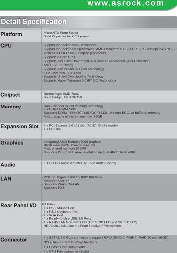
1 x Chassis Intrusion header 1 x CPU Fan connector (4-pin) 1 x Chassis Fan connector (4-pin) 24 pin ATX power connector 4 pin 12V power connector Front panel audio connecto 2 x USB 2.0 headers (support 4 USB 2.0 ports)
