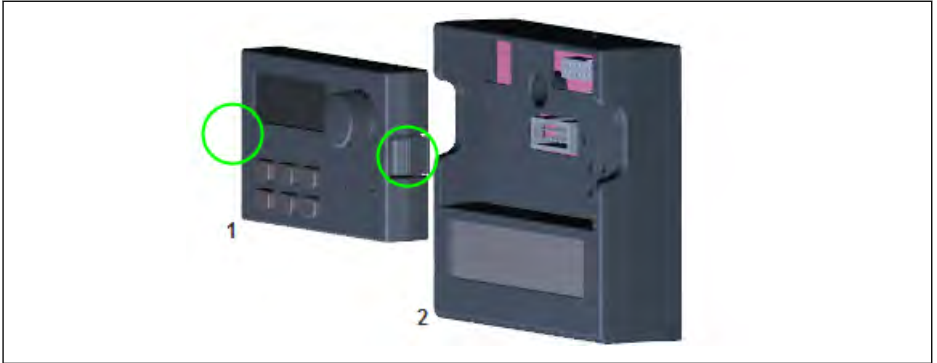
Fig. 17-2: Disassembly of operating panel
