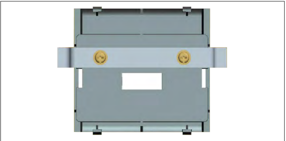
Fig. 16-3: Fix the mounting plate (back view)
