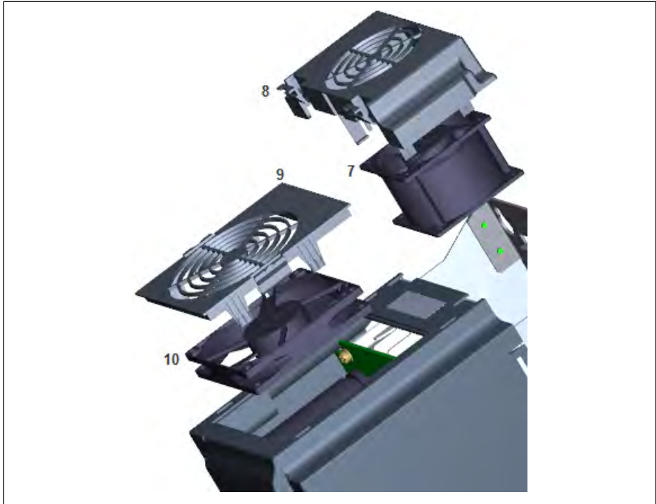
Fig. 17-3: Disassembly of fan
