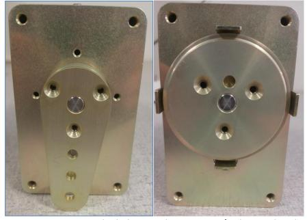
3. Fasten the servo arm or capstan to the hub using the 3 6-32 x 3/8 Flat Head Socket Cap Screws included using a medium strength thread locking compound (e.g. LOCTITE 243). Each fastener should be torqued to 5-7 in-lb.
