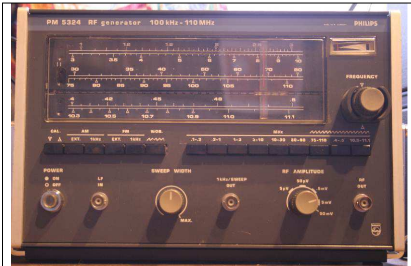
Figure 9 - Philips PM5324 signal generator
