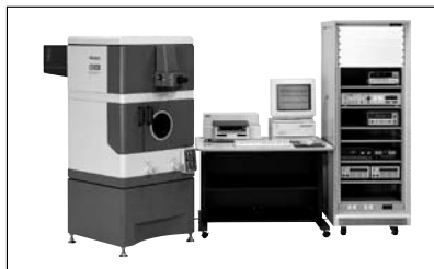
Interferometer used for calibrating gauge blocks (Miyazaki Plant)
