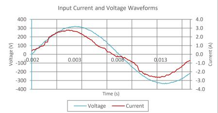
Input AC Current Waveform (ITHD = 15.4%, 50% Load)
