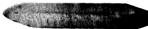
Photo 6 : X-ray topography of a Y-cut containing the seed. Better growth conditions but many dislocations from the seed.
