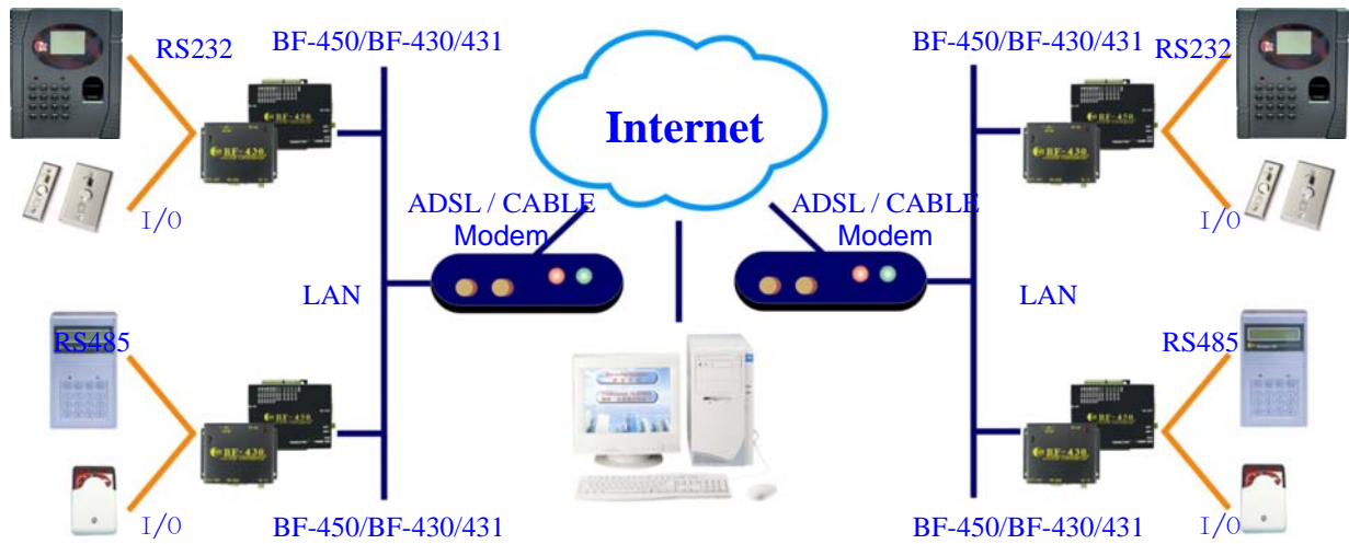
Figure 1 Standalone BF-450/BF-430/431's application through Internet
