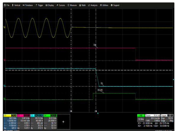
Figure 6: LCC1200-28U-9P Hold-up Time Vin = 264Vac Load: Io = 42.9A (12V), I SB = 1.5A (5V) Ch 1: AC Mains Ch 2: V SB Ch 3: V 0 CH 4: G_DCOK_C
