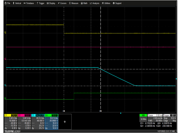
Figure 20: LCC1200-28U-4P Turn Off Characteristic via INH_EN Load: Io = 42.9A (12V), I SB = 1.5A (5V) Ch 1: INH_EN Ch 2: V SB Ch 3: V O CH 4: G_DCOK_C
