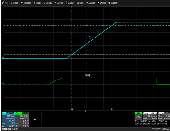
Figure 7: LCC1200-28U-9P Output Startup Characteristic Vin = 264Vac Load: Io = 42.9A (12V), I SB = 1.5A (5V) Ch 3: V O Ch 4: G_DCOK_C
