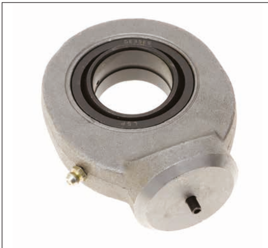
PART NUMBER OTS... AR NOMINAL RANGE 10mm-80mm 3/4"-3" COUPLING SURFACES STEEL /STEEL LUBRICATION REQUIRED
