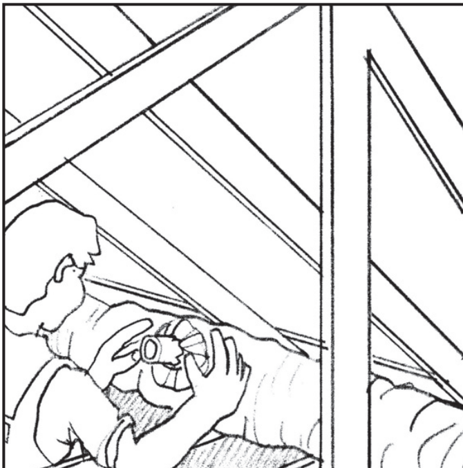
Fig. DUC-11 - BTO with insulation sleeve
