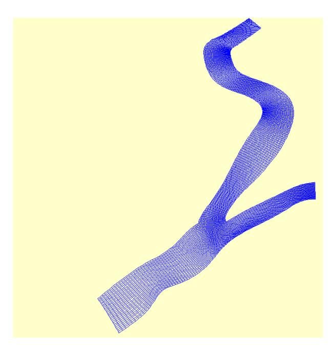
Figure 3.1.J.4 - Computing network on Bala area
