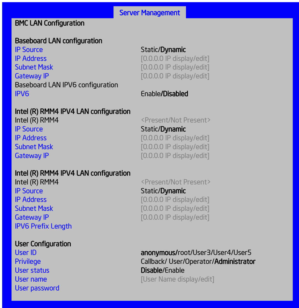
Figure 142. BMC LAN Configuration Screen
