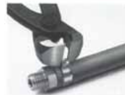
Remove clamp by cutting through outer edge of ear with pincers.
