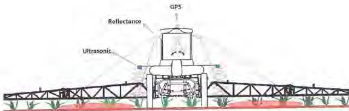
Figure 1. Canopy sensors disposition on a high clearance vehicle.
