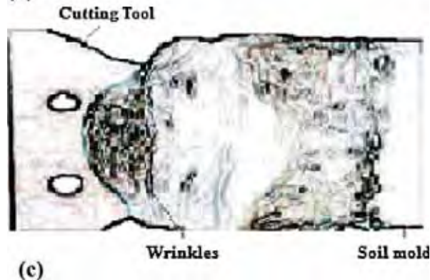
Fig. 7. Flow with considerable bending failure: (a) dry land soil, (b) paddy soil and (c) schematic sketch.
