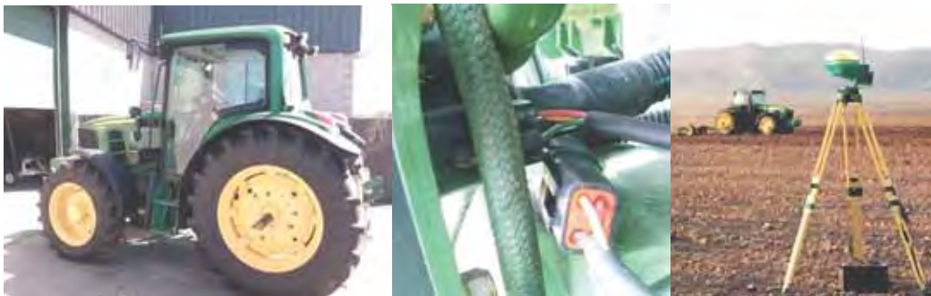
Fig. 4: Experimental tractor (left), CANBUS connection (center) and a base station used to provide RTK-level GNSS signal to determine field elevation.
