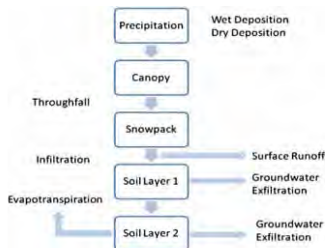
Figure 2 | Definition sketch for the compartments of a watershed (Chen et al. 2001b).
