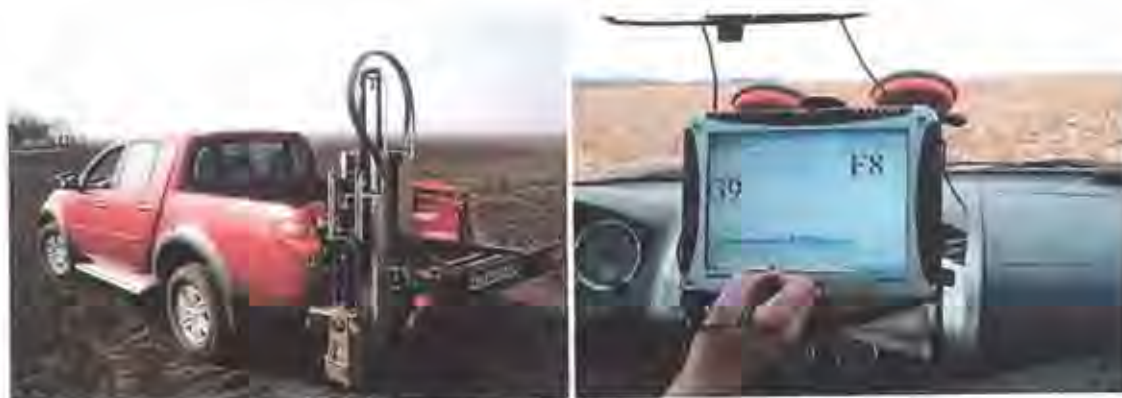
Figure 1. Semi-automated Nietfeld 2005 soil sampling system (left) with in-cab navigation (right) used in this research.
