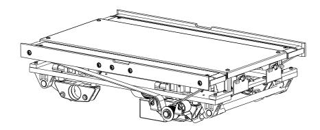
LTUs may be used to direct or accept pallets to/from another LTU via track rollers, to a BS2 transverse conveyor, or to the transport level on a conveyor section.
