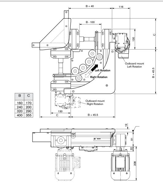
Curve width (B) must match pallet length ( $L_{wT}$ ) or width ( $B_{wT}$ ), depending on orientation.
