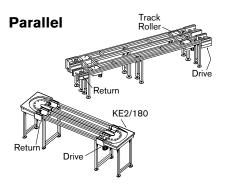
A parallel configuration uses track rollers or KE2/curve units to connect the conveyor sections.
