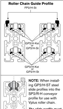
The slide profile must be located in lower position as shown in illustration at left.
