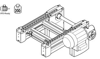
Roller chain transverse conveyors are used to transfer heavy workpiece pallet payloads between parallel conveyor sections. They are also used to construct cycle-independent workstations and are especially suitable for modular system layouts with short conveyor sections at high loads. The unit itself is modular and comes with its own drive, return, and pre installed roller chain.
