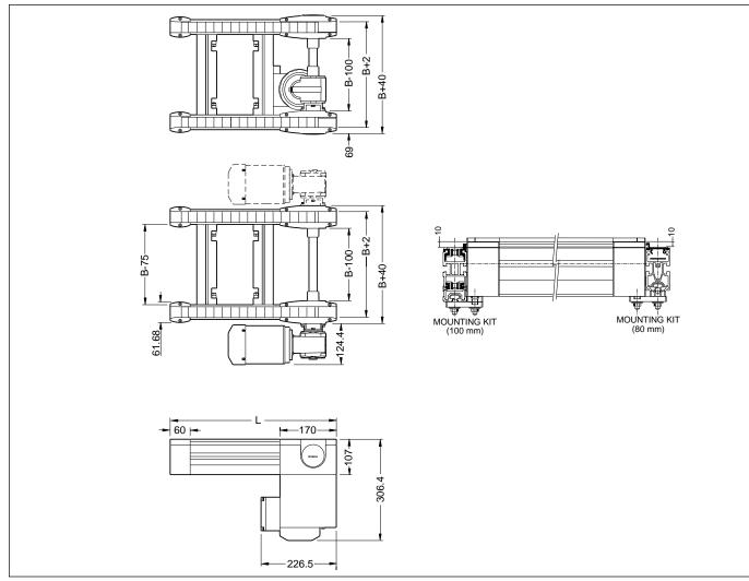
Transverse conveyor width (B) must match pallet length ( $L_{wT}$ ) or width (B<sub>wT</sub>), depending on orientation.
