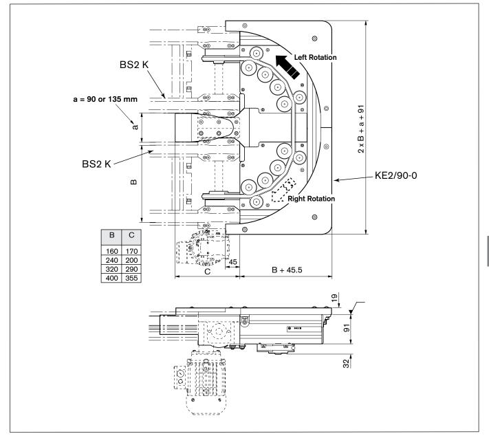
Curve width (B) must match pallet length ( $L_{wT}$ ) or width (B<sub>wT</sub>), depending on orientation.
