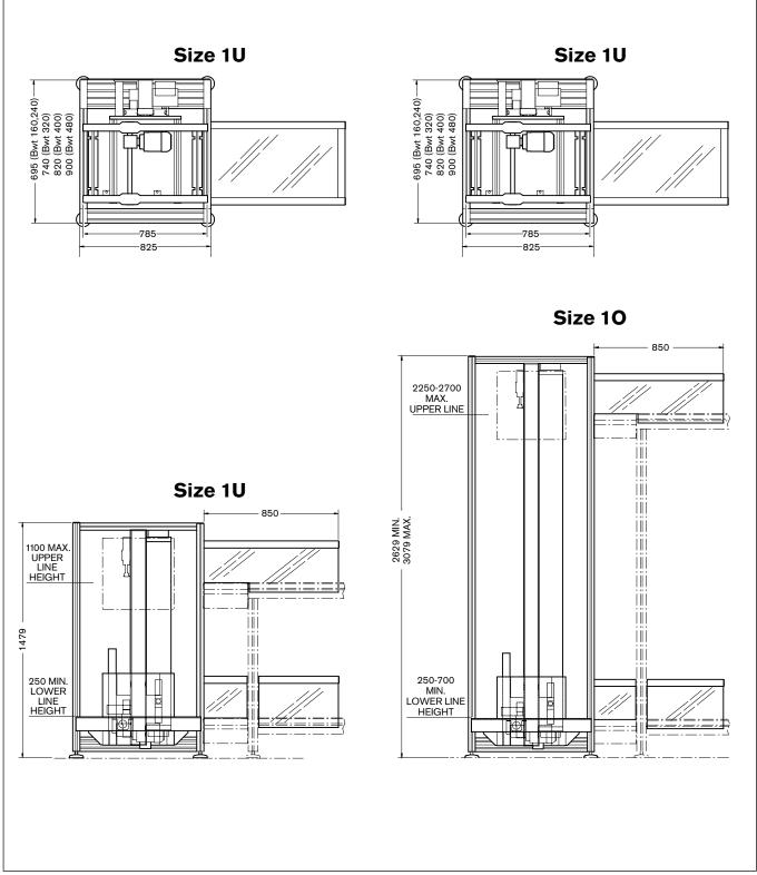
Transverse conveyor width (B) must match pallet length ( $L_{wT}$ ) or width (B<sub>wT</sub>), depending on orientation.
