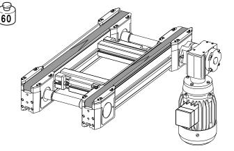
Transverse conveyors are most often used to transfer workpiece pallets between parallel conveyor sections. They are also used to construct cycle-independent workstations, or small systems with short conveying lengths. The unit itself is modular and comes with its own midmount or outboard-mounted drive with toothed drive belts.
