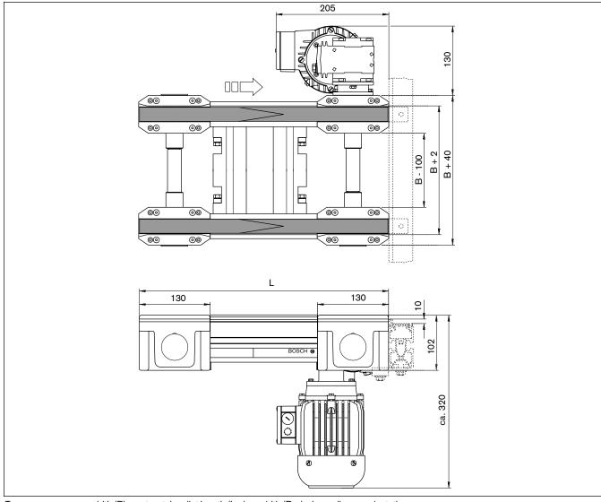
Transverse conveyor width (B) must match pallet length ( $L_{wT}$ ) or width (B<sub>wT</sub>), depending on orientation.
