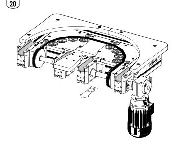
KE2/180 curves have their own drive motor and can be used with most standard TS*plus* drives, returns, and transverse conveyors. Two short toothed belt conveyor segments transfer pallets to and from adjacent conveyor sections.
