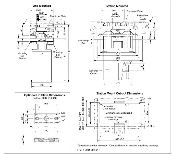
**Note:** Upper end-position damping is only effective when the cylinder's full lift height is reached. Proper guarding must be installed to protect operators when the lift above the chain exceeds 3 mm.
