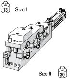
**HP2/K** Lift-position Unit for force absorption 13-10 to 13-14
