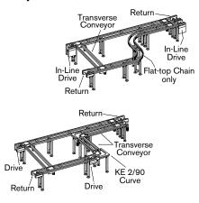
A serpentine conveyor line uses multiple in-line drives and returns, straight conveyor sections, 90° conveyor sections, or 90° curves all connected together by transverse conveyors. Serpentine lines provide the flexibility needed when space or production requirements dictate the need for an unusual layout.
