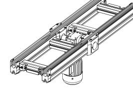
Transverse conveyors are available in any length from 310 mm to 6000 mm in 5 mm increments. Specify conveyor width, length, conveyor speed, motor voltage/ frequency, motor mounting and belt version when ordering.
