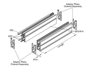
The 10mm T-slot in each side and bottom of the aluminum chain profile allows conveyor modules or peripheral devices to be mounted using T-bolts or T-nuts eliminating the need for special machining.
