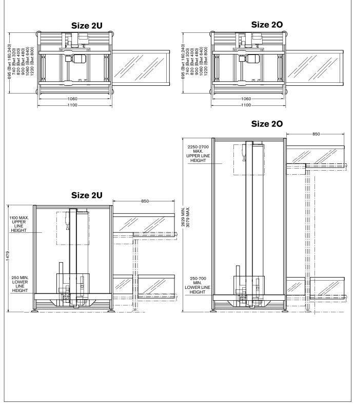
Transverse conveyor width (B) must match pallet length  $(L_{wT})$  or width  $(B_{wT})$ , depending on orientation.
