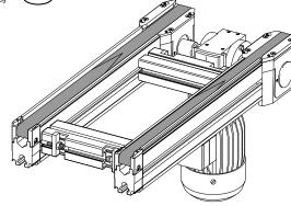
Transverse conveyors come fully assembled and include all required mounting hardware. Motor voltage and frequency options are described in table 9-1.
