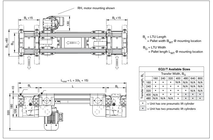
Transverse conveyor width (B) must match pallet length ( $L_{wT}$ ) or width (B<sub>wT</sub>), depending on orientation.
