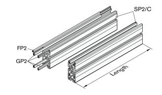
Chain sections can be connected end-toend with connection links to extend the conveyor length (see page 7-1). **Note:** Since leg sets are required at minimum 2 m intervals we stock standard precut 2000 mm sections for quick delivery.
