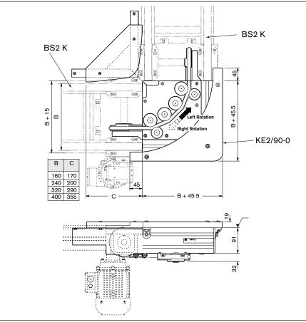
Curve width (B) must match pallet length ( $L_{wT}$ ) or width ( $B_{wT}$ ), depending on orientation.
