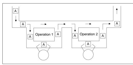
"Cycle-independent stations" can be used to balance assembly operations with differing cycle times.
