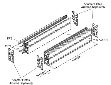
The ST2/C-H section also includes an integrated cable duct on the outside of the profile. This cable duct can be covered with standard 10mm Cover Strip from the Rexroth structural framing product line.
