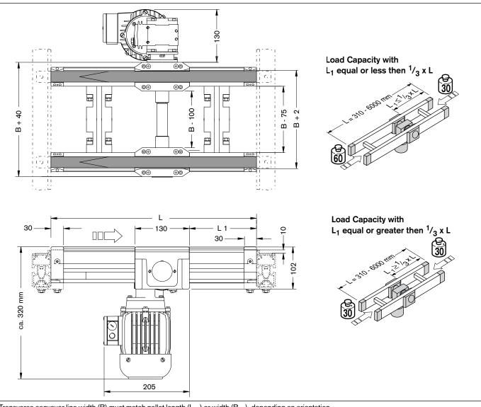
Transverse conveyor line width (B) must match pallet length ( $L_{w\tau}$ ) or width (B<sub>wt</sub>), depending on orientation.
