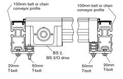
Transverse conveyor width ( $B_{wT}$ ) must match pallet length ( $L_{wT}$ ) or width ( $B_{wT}$ ), depending on orientation.
