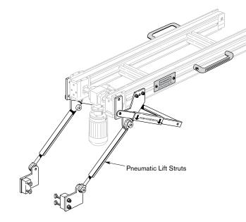
Lift gate kits are available in pallet widths from 160-800 mm, and two different pneumatic lift struts are used depending upon BS2 length. Standard lift struts handle BS2 conveyors in length ranges of 1010 to 1310 mm while high capacity lift struts are used for BS2 conveyors in length ranges of 1315 to 1610 mm. Lift gate kits can be mounted in any of the four basic configurations shown on page 9-5.
