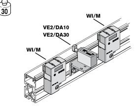
an economical means of softly stopping pallets traveling along a transverse conveyor section.
