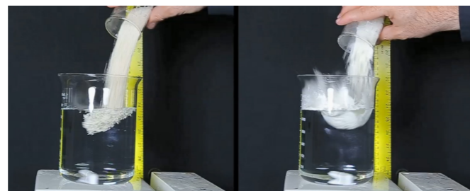
Polyclar™ Brewbrite Granules (left) and powdered product (right) added directly to liquid.
