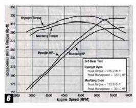
or a variable load that maintains a preset engine rpm or vehicle speed. This feature is ideal for forcing the vehicle to operate at certain loads for tuning. The Dynojet can also measure air/fuel ratio while testing.
