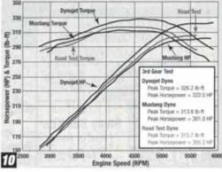
dynos. You can also see that the Dynojet dyno measures a higher rear-wheel horsepower than the Mustang dyno. The Dynojet measured 5.1 percent higher horsepower in Fourth gear, 7 percent higher horsepower in Third gear, and 8.2 percent higher horsepower in Second gear. We will try and explain this difference a little later.
