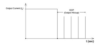
It is not recommended to prolong the duration of  $I_{\rm O}$  when it is <110-150% but >100%, since it may cause damage to the PSU.
