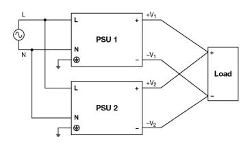
Fig. 4 Parallel Operation Connection Diagram
