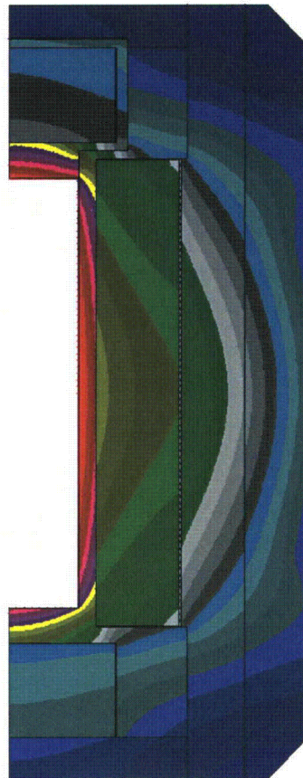
Figure 3-129. Load Case 115 – Fire at 150 Minutes, 100°F, Maximum Decay Heat, Maximum Insolation, Cask Model – Model AOS-165
