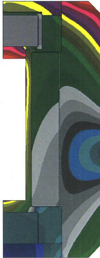
Figure 3-97. Load Case 113 – Fire at 90 Minutes, 100°F, Maximum Decay Heat, Maximum Insolation, Cask Model – Model AOS-025
