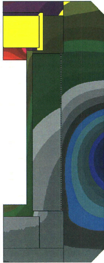
Figure 3-99. Load Case 114 – Fire at 120 Minutes, 100°F, Maximum Decay Heat, Maximum Insolation, Cask Model – Model AOS-025
