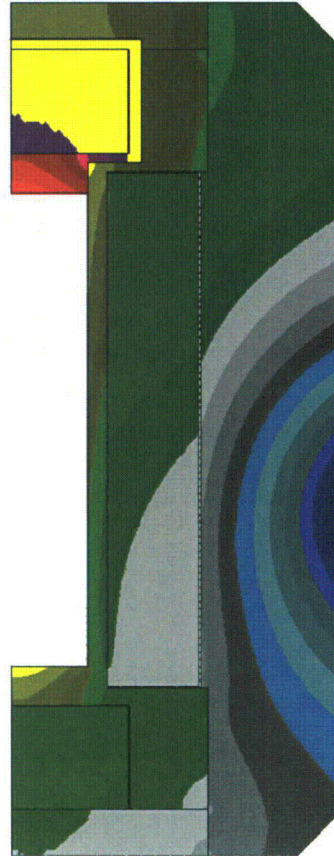
Figure 3-103. Load Case 116 – Fire at 180 Minutes, 100°F, Maximum Decay Heat, Maximum Insolation, Cask Model – Model AOS-025
