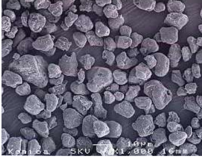
Traditional Resin Toner Particles
