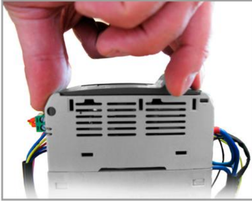
1. Open fuse holder by pulling the frontal cover
