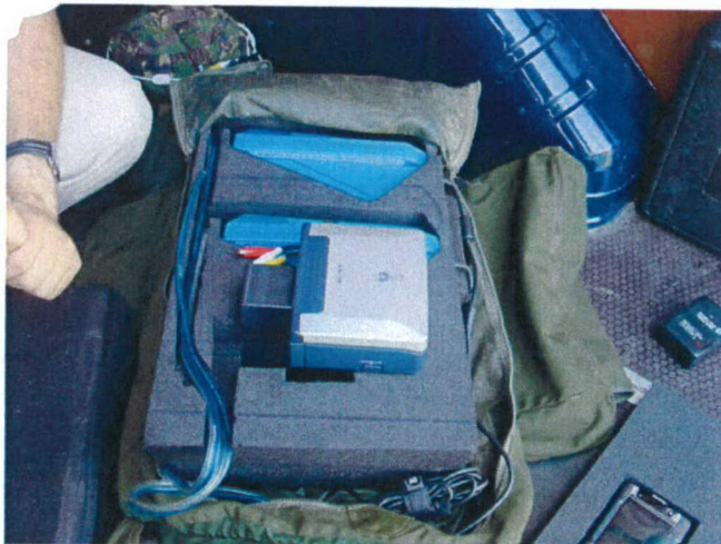
Figure 2 Photo of the new system which comprises of two Portacounts, which are individually coupled to data loggers. Also visible is the portable video-recorder which is fitted to a camera, which on its turn is placed on the helmet.
