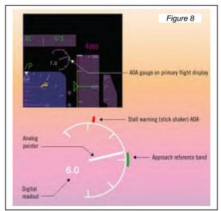
Many AOA indicators used in the past have been of the "normalized" type, where AOA is shown in arbitrary units and scaled so that zero load factor is shown as an AOA of zero and stall is shown as an AOA of one. Normalized AOA on a commercial jetliner would require that Mach number be introduced into the calculation of AOA because stall AOA and buffet margins are a function of Mach number.
