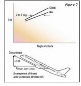
The examples cited above show that many parameters affect the relationship of lift and AOA. For AOA information to be useful to a flight crew, these parameters must be considered and accounted for in the indications and associated crew procedures.
