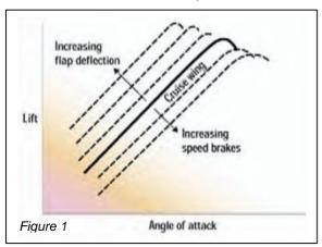
However, many other parameters influence the lift that a wing produces. The most basic is the configuration of the wing, specifically the position of the trailing-edge flaps, leading-edge flaps or slats, and spoilers. As the trailing-edge flaps are extended, the curvature (or camber) and area of the wing are increased, and the wing will produce more lift at the same AOA. (see *figure 1*)
