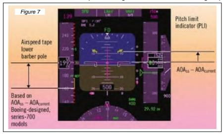
PLI shows AOA margin to stall warning, even though it is part of the pitch attitude display (see figure 7). The distance from the airplane PLI symbol to the calculated from the difference between the AOA of the airplane and the AOA at which stall warning will provides occur. This flight crew with good situational awareness. enabling them to monitor airplane attitude in pitch and
