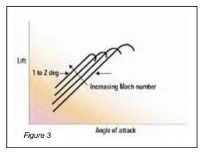
However, higher Mach reduces the maximum lift the wing can attain and the AOA at which stall occurs. This means that as gross weight, altitude, or load factor is increased, the
