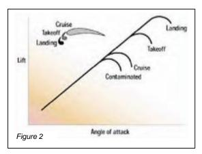
Figure 2 illustrates this and the effect of contamination, such as ice or dents, on the leading edge. Contamination can cause the airflow to separate at a lower AOA, causing the wing to stall at a lower AOA than expected. While these effects are accounted for in the airplane design and maintenance program, it is important to remember this potential variability in stall AOA.
