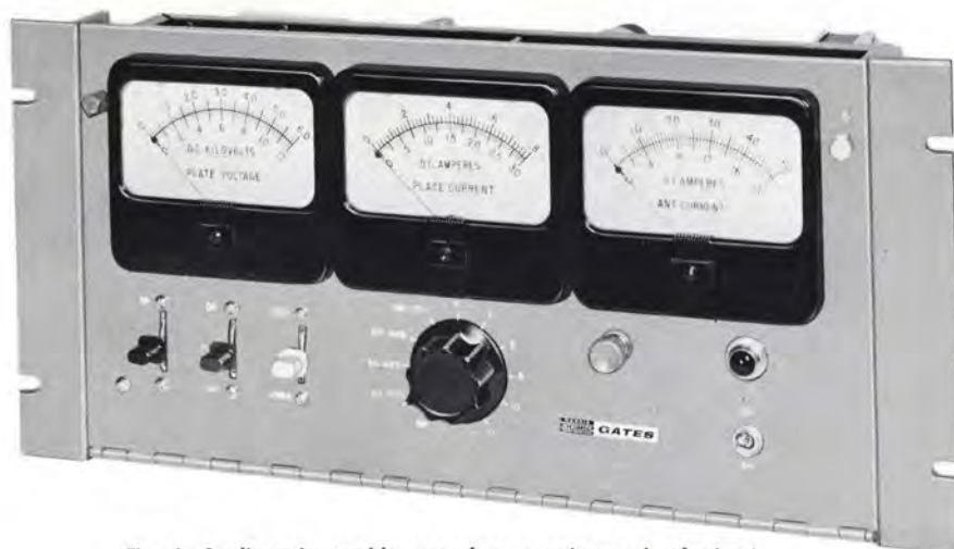
Fig. A. Studio unit provides complete metering and selection/operation of up to 23 control functions. Power supply is self-contained.
