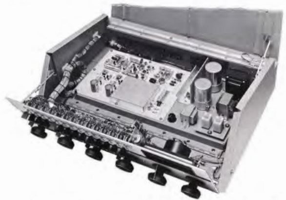
Hinged top cover and front panel swing open for easy access to components.
