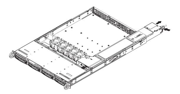
Figure 6-6. Removing/Replacing the Power Supply
