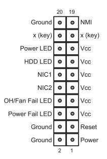
Figure 5-3. Front Control Panel Header Pins (JF1)
