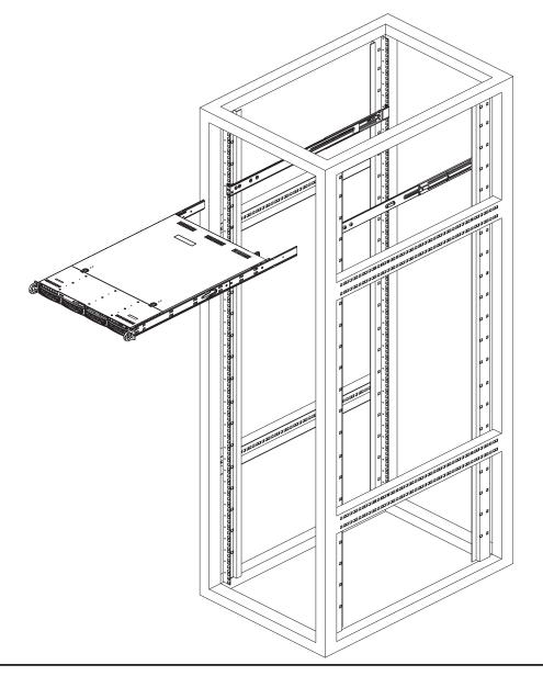
Figure 2-3. Installing the Server into a Rack
