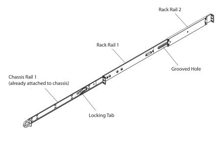
Figure 2-2. Installing Chassis Rails
