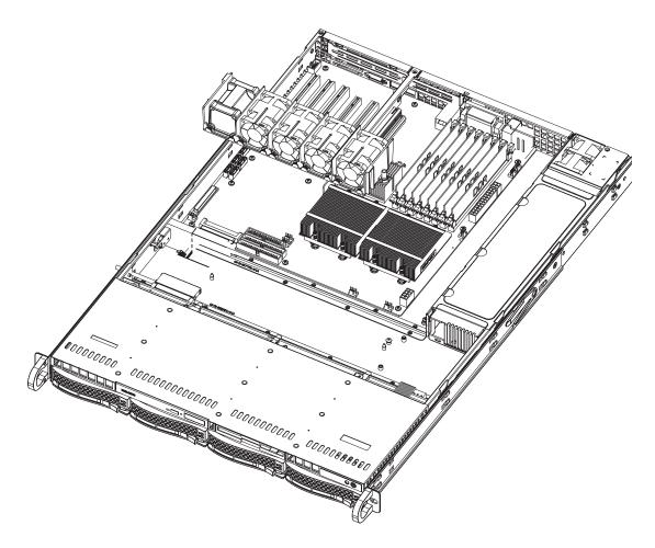
Figure 6-2. System Cooling Fans
