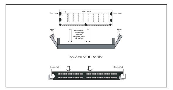
To Install: Insert module vertically and press down until it snaps into place. Pay attention to the bottom notch.
