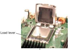
CPU installed in socket
