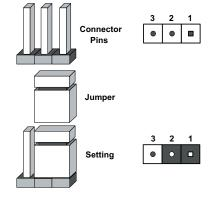
**Note:** On two-pin jumpers, "Closed" means the jumper is on and "Open" means the jumper is off the pins.
