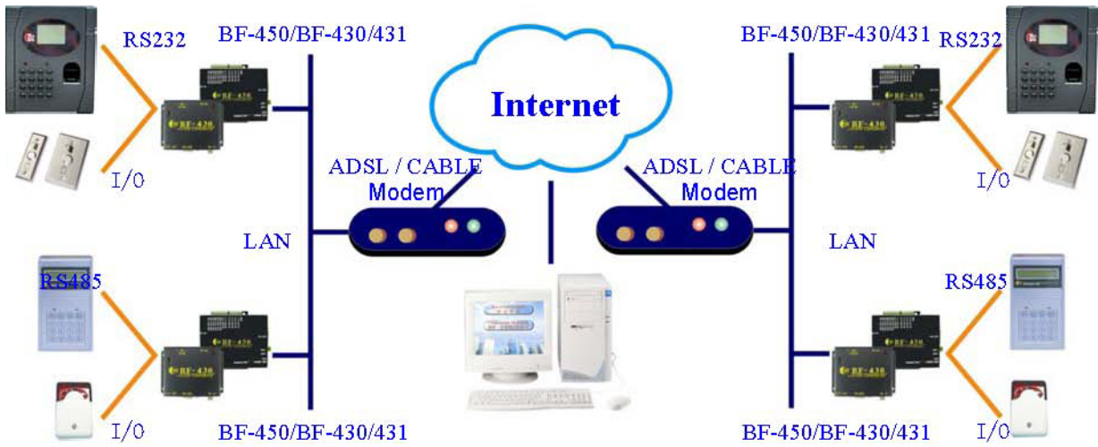
Figure 1 Standalone BF-450/BF-430/431's application through Internet
