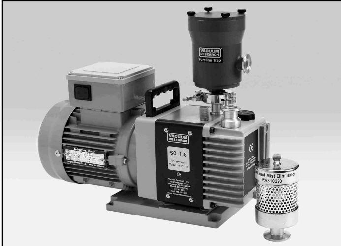
Photo shows Pump with optional inlet trap installed and exhaust mist eliminator. See pages 14 and 15 to order these accessories. Power on/off switch, resettable circuit breaker and line cord are standard on pumps shipped with single phase motors.
