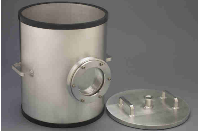
12 inch cylinder with 'L' gasket, optional Pyrex view port, handles, and top plate. Less outgassing than stainless steel, see page 39.
