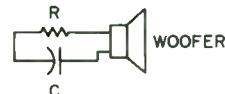
FIGURE 4: If you use a passive crossover, an impedance-compensation network can help you maintain a constant 8Ω impedance. See Table 2 for component values.
