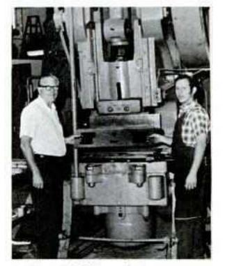
DOC ULRICH, plant manager (left) and an employee hold a piece of metal formed in the 110-ton punch press behind them. The huge machine, part of a complete metal working section, costs \$30,000.
