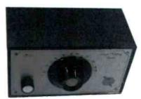
MILLER TUNER - The Miller Coil Co. produced this high fidelity tuner in 1956. It is a crystal set using sophisticated Miller coils which can separate stations better than most other sets on the market. It sold for \$14 in kit form or \$19 factory-built. (Fred Geer - Jacksonville, FL 32210)
