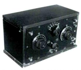
Figure 1. The Tuska Model 224 Receiver. Notice the small metal hooks used to hold the cover lid closed.
