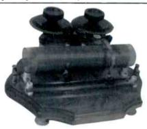
UNIQUE HOME BREW - This is a Hugo Gernsback Detectorium of 1910 design. The crystal is mounted in a cup that makes direct contact with the wire on the rather long coil, sliding up the coil for tuning. Another slider, on the left, controls the length of the coil. This unusual home brew tunes long wave and shortwave, and even today its owner claims it will pick up Radio Moscow and the BBC. (Fred Geer - Jacksonville, FL 32210)
