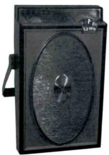
ZENITH ROYAL 500H DELUXE - This 1962 radio had a 5x3-inch speaker with a ceramic magnet and an off-center voice coil, which makes it sound very good. It came in three colors, had four tuned IF circuits, 200 milliwatts undistorted audio output and vernier tuning. It sold for \$60. (Fred Geer - Jacksonville, FL 32210)
