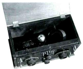
Figure 2. Interior view of the Tuska Model 224 showing the tube placement and the molded tickler coil to the right.
