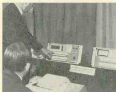
Exciter-modulator of new Gates uhf television transmitter (320) pulls out for testing.
