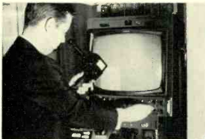
Top, new programmable signal generator for testing CATV headend from Tektronix (338). Bottom, the Gardner Colorgard meter (339) for matching monitors at 6500K at the Television Equipment Associates booth.
