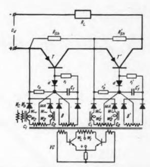
Fig. 3. Control circuit for series-connected transistors has square-wave base pulses supplied by magnetic amplifiers. Shunting resistors  $R_{ah}$ ,  $R'_{ah}$  equalize transistor voltage for cut-off condition.
