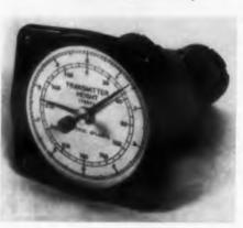
Series IU dual synchro position indicators are designed for accurate, non-ambiguous indication of linear or angular position of transmitter units. The indicators can be read accurately within ±0.03 deg from a 5-1/4 in. panel mounting. A separate synchro receiver is geared to each pair of concentric dial pointers. Model IU-3 indicator can be reset to zero with respect to an arbitrary reference point; Model IU-6 indicator monitors mechanisms with fixed reference points.
