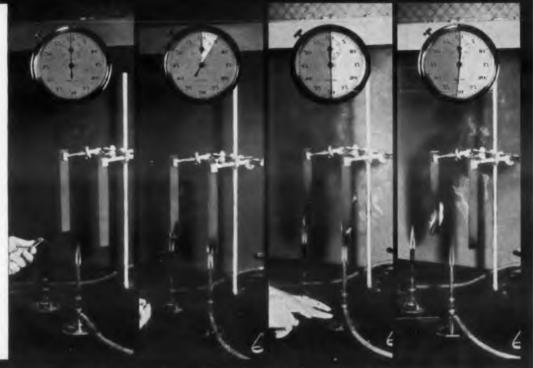
Actual flame test of a non self-extinguishing glass-epoxy laminate and Textolite G-11 (11559) glass-epoxy laminate. Less than two seconds after removal of burners, flame on 11559 dies, the other glass-epoxy laminate continues to burn.
