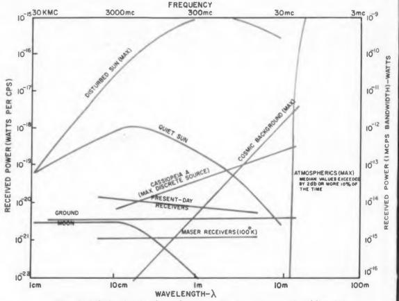
Fig. 5. Relative levels of interference noise power across the rf band due to radiation encountered in space.
