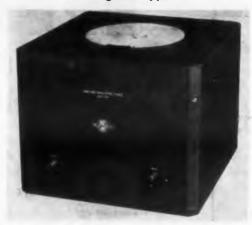
Model 61A angular oscillating table is for frequency-response testing of gyros, accelerometers, and guidance systems. A rate pickoff provides instantaneous rate information for presentation on an oscilloscope or recorder. Input may be from any audio amplifier, de power amplifier, or shaker amplifier over the range of 0 to 100 cps.
