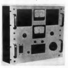
The Model HC 36-50 transistorized power supply is rated at 0 to 36 v from 0 to 50 amp dc, and has a line regulation of 0.05% and a load regulation better than 0.1% for 0 to full load changes. Ripple is less than 2 mv. Input power is 208 v, 60 cps, 3-phase, four-wire wye. The bias supply, amplifier and overload circuitry are contained in separate plug-in modules. Dimensions are 17.5 x 20 x 19 in. for rack mounting.
