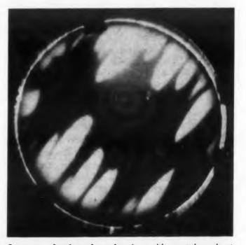
Superconductive domains in a thin tantalum sheet appear as dark areas. Magneto-optical technique developed by Dr. Warren DeSorbo at GE Research Laboratory permits direct visual observation of intermediate superconductive state. Normal areas shown in white, are elongated in the direction in which the sheet was rolled.
