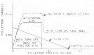
Fig. 2. Binistor E-I characteristics with varying input bias conditions.
