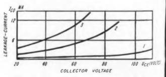
Fig. 2. Since the leakage current-collector voltage relationship varies between units, the source voltage will not divide equally when the transistors are cut off.
