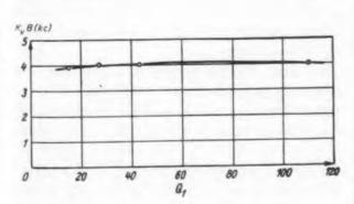
Fig. 4. Gain bandwidth product as a function of signal tank Q.
