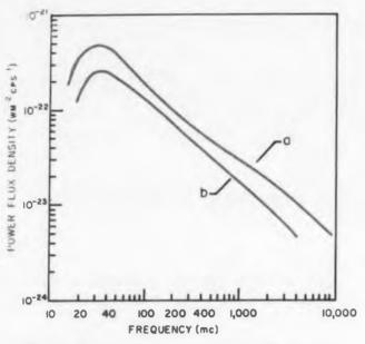
Fig. 3. Power spectra associated with the two most intense discrete sources detected to date (a) Cassiopeia A and (b) Cygnus A.
