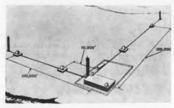
L-shaped receiving station network planned for missile trajectory measurements over the Atlantic Missile Range. The central station along with either the pair of receiving stations 10,000 feet away or the pair 100,000 feet away provides a point position for a missile. Errors are expected to be small in relation to missile size.
