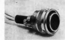
The KQ/KR Series connectors consist of Type KRO receptacle, Type KQ ball-lock plug, shown, and Type KR bayonet-lock plug. These crimptype, miniature plugs have removable snap-in contacts. The receptacle will accommodate either the ball-lock or the bayonet-lock plugs. Plugs with 3 to 55 contacts and ratings from 1250 to 2400 v are available. The series has been tested to 100,000 ft and at 257 F.
