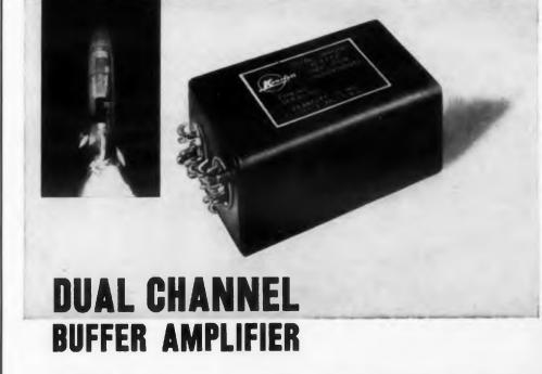
This small, light-weight unit, a completely transistorized dual channel buffer amplifier, is designed to drive Kearfott's size 11 R980 winding compensated synchro resolvers. The amplifier-resolver combination has stable gain characteristics and negligible phase shift through an ambient temperature range of —55°C to +85°C. This unit meets the environmental requirements of MIL-E-5272.
