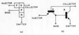
Fig. 1. (a) Physically the silicon binistor resembles a four-layer switch. (b) Equivalent circuit for the binistor.
