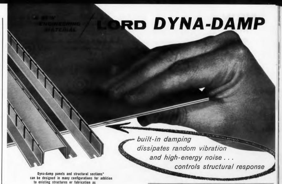
Lord announces Dyna-damp—a new engineering material that counteracts broad-band "white" noise and vibration. It offers a new, better way to solve acoustic fatigue and structural response problems.
