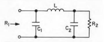
Fig. 1. This pi-network can be easily designed using the equations given in the text.
