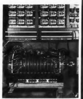
Magnetic drum memory of package sorter. Destination of packages traveling on pallets is written on drum by operators. When package is above its destination bin, command is given for the pallet to tip the package into the bin.
