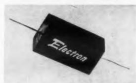
Series DE capacitors are available from 0.001 to 0.68  $\mu f$  in 200, 400 and 600 vdc values. Made with metalized Mylar, the units are encased in epoxy tubes. Operating temperatures are -55 to +85 C; insulation resistance is 10,000 meg; dissipation factor is less than 1% at 25 C. The 0.001 to 0.033  $\mu f$  units measure 0.57 x 0.29 x 0.17 in.
