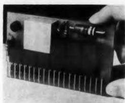
These magnetic shift registers, offered in 5-, 9and 10-bit modules, use only one core per bit. Each module contains its own shift drive, widewidth gate, and hold-gate circuitry. Model 9TDWW150/U, shown, is a 9-bit unit with a maximum frequency of 150 kc and an input-output pulse of 6 v. Typical applications are in short
