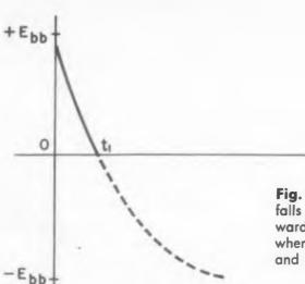
Fig. 5. Voltage  $V_{EB2}$  falls exponentially towards  $-E_{bb}$  until  $t_1$  when  $Q_2$  turns "on" and  $Q_1$  turns "off."
