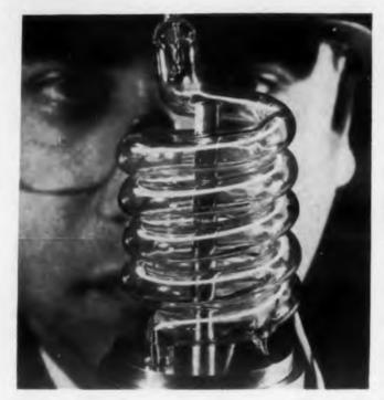
**Hughes laser** shown without housing consists of ruby cylinder surrounded by high intensity mercury discharge lamp. Interferometer necessary for operation can be achieved by mirroring ends of the cylinder or by mirroring the end plates of the laser housing.
