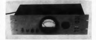
The Type TR-942-C volume level indicator is a transistorized version of the Series 924 indica-
