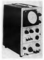
Model S42 high-writing-speed oscilloscope uses a 4-in. cathode ray tube. Operating at 3.7 kv, it provides a brightness so that a 1-usec, single-shot pulse can be seen and photographed. Balanced low-drift amplifiers have a bandwidth of dc to 6 me up to 100 mv per cm. Gain is 10 mv per mc. Features of the S31 that are retained include time and voltage calibration with built-in squareway calibrator and automatic sync and selective trig ering. Maximum speed is 0.1 usec per mc. The unit weighs 18 lb.
