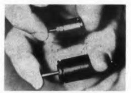
This size 5 gearhead and speed reducer unit weighs only a few grams; it measures 3/4-in. long and is 1/2-in. in diameter. It can have step-up or step-down ratios from 10:1 to 2,025:1. It is designed for satellite applications.
