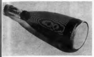
Model K1931 5.25-in. cathode-ray tube is for high-frequency operation for general purpose oscilloscopes and other instruments. The tube has inear post-acceleration for use in low-frequency instruments. It operates at screen voltages of 5.000 v with deflection factors of 25 to 35 v per in, for both sets of deflection plates.
