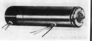
This motor-integrating tachometer, size 10, has a diameter of 0.937 in., a rotor moment of inertia of 3 gm-cm<sup>2</sup> and an acceleration at stall of 9,500 radians per sec<sup>2</sup>. The scale factor is 2.5 v per 1,000 rpm and the linearity from 0 to 3,600 rpm is ±0.12%. Temperature range is -55 to +125 C. The device is suitable for use in analog computers and velocity regulation systems.
