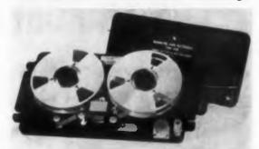
Wideband multi-channel recording under rugged environmental conditions is the primary application for the Model PMR-300 tape recorder. The unit measures  $10 \times 6 \times 4-1/2$  in., weighs 4-3/4lb and requires less than 18 w from a 24-v dc source. Recording bandwidth is 100 kc at 30 ips, and lower speeds with proportionately reduced bandwidth are available. Modular electronic circuits for up to seven channels on 1/2-in. tape are available.
