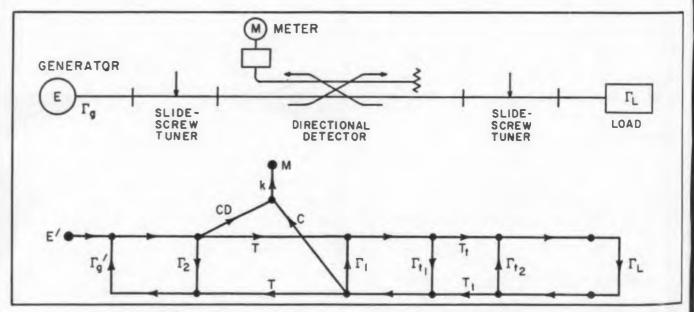
Fig. 4. Equivalent flowgraph of a single-coupler reflectometer used to measure load-reflection coefficient.
