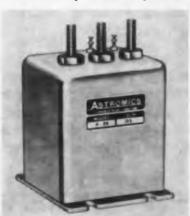
Type A-2A relay is a non-magnetic latching unit that mechanically locks in either the open or closed position, and requires a new command pulse before it can be reactivated. Contacts are plug-in type, assuring contact under extreme conditions and permitting loads up to 20 amp at 26.5 v dc. Energizing current is 0.25 amp at 18 to 32 v dc.
