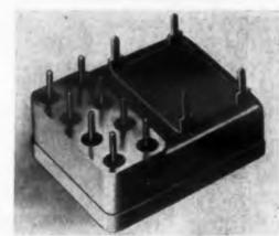
Style 6A dpdt relay is similar to the firm's style 6 relay but is smaller. Installed height is about 0.44 in. Terminals and mounting tabs conform with the 0.2-in. grid pattern. The unit operates at coil powers lower than those required for larger current-sensitive relays in the same class. It switches load currents of 2 amp resistive and higher at 26.5 v dc or 115 v ac. It stands 50 g shock and 20 g vibration at 2,000 cps.
