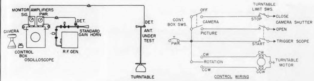
Fig. 1. Antenna beam-width-recorded circuit is built from standard test components.
