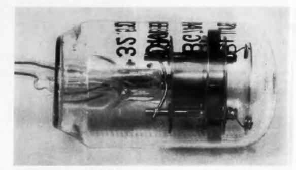
**Rugged 3-mc quartz crystal** produced by Bliley Electric Co., Erie, Pa., for Transit satellite. Crystal is designed for minimum temperature coefficient.
