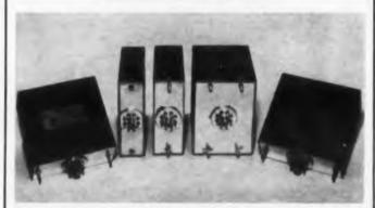
These transistor-regulated power supplies are 1.25 to 1.5 in. wide, depending on power output. Depth and length are both 4 in. Designated the 7400 series, the units are rated at 5 to 60 v dc at 200 ma. No load to full load regulation is 0.05% and line change regulation is ±10%. Ripple is less than 2 mv.
