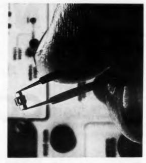
**Unpainted unit** glows with red-heat as 10-amp current is sent through it.
