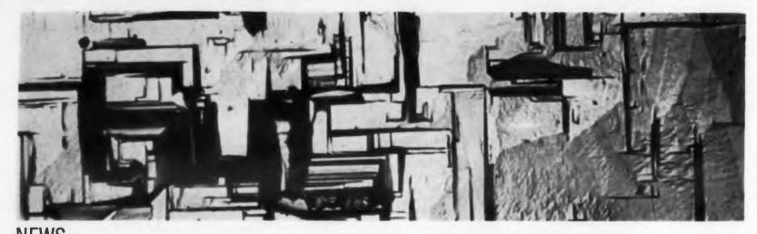
the exotic design at left is representative the exotic circuits that may be positive using the epitaxial-growth process—position of vaporized silicon so that it at tinues the single crystal structure of seed crystal. This is an example of silic deposition on a crystal oriented along 100 plane.
