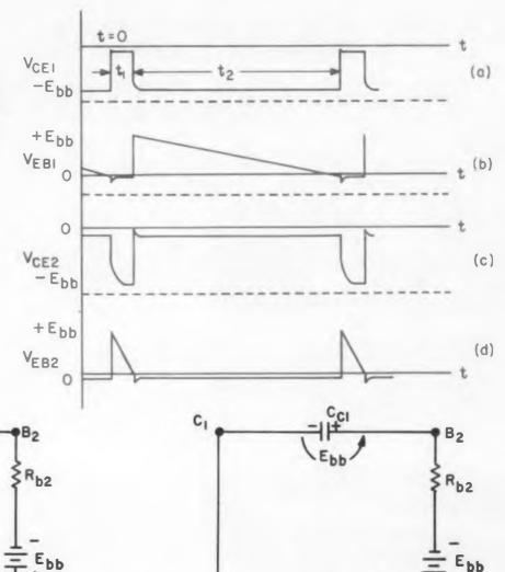
lectors, the transistors should be saturated when in the "on" or conducting state. Then the collector voltage will vary between  $E_{bb}$  and zero volts (actually about 0.3 v).
