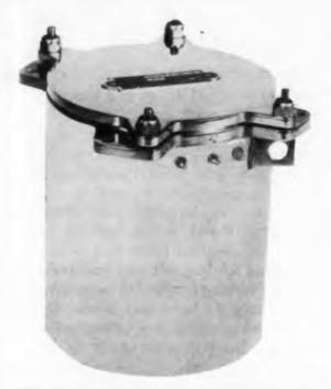
This Dewar flask is used to maintain a stable temperature for the stable oscillators in the Transit program. The quartz crystal is mounted in the flask, and the oscillator circuitry is mounted on a circular plastic board fitted inside the top of the flask.
