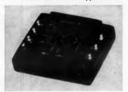
The Model 1806 demodulator-phase detector is designed for guidance applications in missiles and aircraft. The unit provides a dc voltage proportional to the amplitude difference between the signal input and reference input. Frequency response is 700 to 15,000 cps. The device is encapsuled in epoxy resin.
