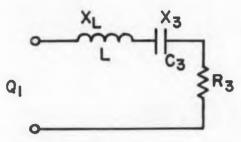
Fig. 3. The value of inductor L, placed in series with  $R_3C_3$ , is calculated from Eq. 3.
