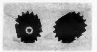
The Model 3AL-685 radiator, designed to prevent thermal runaway, has an 8-32 tapped-stud hole for mounting all transistors having TO-31 and TO-26 packages. Radiators, designed for mounting on printed circuit boards, have two mounting pins 0.3 in. apart. They are 1/2 in. long with 1/2 in. in diameters. Units have 15 cooling fins for a total of about 4 sq in. of radiating surface
