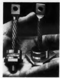
These Quad-Sealed silicon rectifiers are rated from 45 to 150 amp at 50 to 600 v over a temperature range of -20 to +130 C. They can withstand surge currents of 1000 amp peak. They are recommended for industrial power and battery charging applications. Stud mounted, flat base and reverse polarity types are available.
