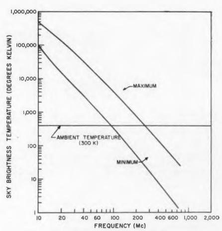
Fig. 2. Maximum and minimum levels for observed cosmic background radiation or continuum; equivalent black body temperature plotted vs frequency.
