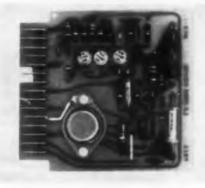
These solid-state transistorized modules are rated at medium speeds of 200 kc and high speeds of 3 mc; the magnetic types are rated at medium speeds of 50 kc and high speeds of 100 kc. Transistorized NOR logic modules and high-temperature modules are also available. All modules have 15-pin connectors.
