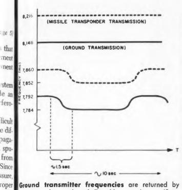
Ground transmitter frequencies are returned by a transponder on the missile with a continuous 68-mc offset. Beating the high and low carriers together gives a 256 mc if which is swept down to 264 mc over a 1.5sec interval. The sweep returned from the missile is offset in time from the ground transmitter frequency sweep by a few milliseconds—corresponding to the signal transit time. No measurements are made on the 8 mc upsweep, used to maintain phase-lock throughout
