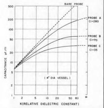
Fig. 2. Capacitance of insulated probes is a nonlinear function of the dielectric constant of the insulating sheath.
