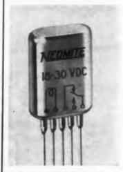
Encased in transistor can
