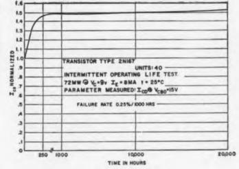
The rate-grown process produces a small, clean junction which exhibits almost no drift or deterioration at high voltages and offers the user low  $I_{\rm CO}$  and  $I_{\rm EO}$ . Two new types, the 2N1510 and 2N1217, will be useful for low-level switch and neon indicator applications. Both the 2N1217 and 2N167 operate at extremely low current and leakage levels, making them ideal for starvation circuits of 2 ma or less.
