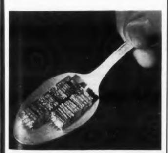
Technician removes micromodule flip-flop from the navigation computer used with the RCA micromodularized inertial-guidance system, upper and lower left. Pencil at lower left points out some of the preamplifier micromodules, which have been mounted on the inner gimbal of the guidance system to cut down on the number of slip-rings required. Size of encapsulated modules is illustrated above. This spoonful is equivalent to sin-transistor commercial receiver.
