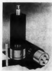
Types ST-9 and ST-10 silicon plug-in rectifiers directly replace types 8008 and 872A mercury vapor rectifier tubes respectively. The units are rated at 10,000 piv and 1,250 ma dc output. Temperature range is from -65 to +75 C. The rectifiers are hermetically sealed. The ST-9 measures 8.03 in. x 2.13 in. diameter; the ST-10 measures 8.18 in. x 2.31 in. diameter.
