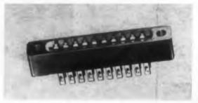
Series 600 printed circuit connectors accept 1/32-in. printed circuit board or tape cable. A double row of 10 contacts with solder lug terminals provides 20 connections for board and circuit wiring on a connector length of 1-7/8 in. Voltage ratings are 650 v rms at sea level, 200 v rms at 70,000 ft. Current rating is 3 amp.
