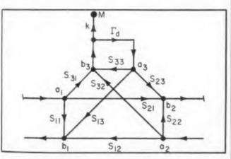
Fig. 3a. Three-port network terminated by a detector.
