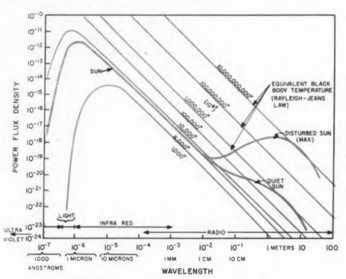
Fig. 4. Solar power spectra observed on earth.
