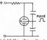
G-E NE-77 in a Trigger Circuit
