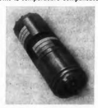
Model 15A23D-O1C motor tachometer is a precision temperature-compensated, non-frequency sensitive instrument. Output is 2.75 v per 1,000 rpm  $\pm 0.25\%$  from 0 to 70 C, with adjustability to  $\pm 0.01\%$  from 60 to 80 C. Linearity to 3,600 rpm is within  $\pm 0.07\%$ . The unit is designed for missiles, computer packages, electronic systems and airborne or ground support control units. Environmental Mil specs are met.
