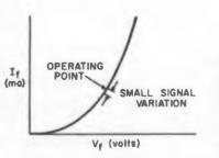
Fig. 2. Small signal operation of diodes keeps their forward resistance almost constant in the operating range.
