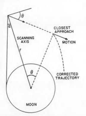
**Retro-rocket** applies impulse to give the desired corrected trajectory at the closest point of approach to the moon. The rocket is positioned so that its thrust is opposite to the motion at the correction point. Tracker measurements will indicate dr/dt = O;  $d\Theta/dt = \max d\alpha/dt = O$  at the correction point. Known radius of the moon times  $\csc \alpha$  results in the r measurement.
