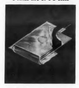
Cathodic Envelope design doubles anode and cathode areas to give high current, low impedance required for transistor circuits, provides volume efficiency unknown to other carbon zinc cells with no side penalties for peak performance!
