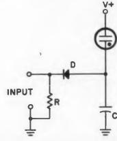
Capacitor C holds the fast input pulse voltage amplitude until the neon tube can fire.
