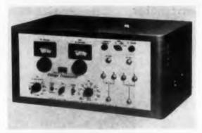
Models VC-12 voltage comparator provides simultaneous dc and rf voltage reference traces on the sweep frequency display. The unit is made up of three sections. A switch contains two spdt, coaxial, mercury relays having a vswr of less than 1.1 from dc to 250 mc. An rf section has a calibrated 1-mc signal that may be varied from 120 uv to 12 v rms. A dc section has positive and negative outputs of 120 µv to 12 v.
