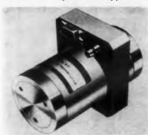
The Model 571 altitude control transducer is economically designed for use in expendable target drones or tactical missile and aircraft applications. The unit employs a trapped-air-pressure design to provide an accurate altitude error signal. It operates to 80,000 ft with a dynamic error band of  $\pm 2\%$ . Functional range is  $\pm 0.5$  psi. The unit has a  $2 \cdot 1/4$  in. diam and is  $4 \cdot 1/4$  in. long.
