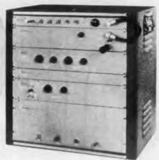
This unit features an electronic pulse delay that can be set to zero or is continuously variable from .030 microseconds to 500 microseconds in five ranges. Pulse width is continuously variable from .02 to 12.5 microseconds in four ranges.
