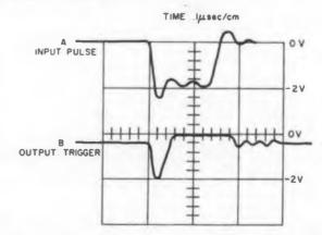
Fig. 2. Sketches taken from an oscilloscope show the 0.2-µsec input pulse (a) and the resultant 0.05-µsec output pulse (b).
