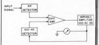
**Linear readout results** from nonlinear detection of incoming rf and 100-kc signal.
