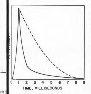
latural fluorescence time in ruby is reduced from apparential decay curve to sharp peak.
