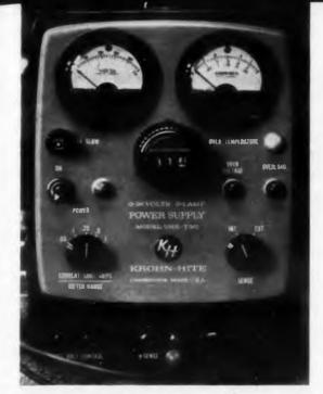
Bench-model supply has digital voltage dial, accurate to 50 mv. The dial is also featured on rack-mounted units.
