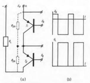
Fig. 1. Voltages higher than the individual transistor's rating can be switched by connecting two transistors in series.
