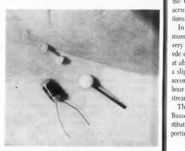
Blood flow meter components shown here are too large for animal or human use. The 6-mm ball was used in simulated flow experiments. Both the magnet coil and its plastic bobbin are illustrated. The ball is machined of Teflon or other physiologically inert material.
