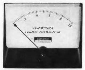
A NEW INSTRUMENT measure switching times as short as half a nanosecond. Five times faster and to times more accurate than earlier instruments that did part of its job, this test measures rise, fall, turn-on, turn-off, and storage times, one at a time or in an sequence.
