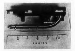
Suited to operate in series as an amplifier chain, types L-3266 and L-3236 PPM-focused traveling wave tubes cover 7,000 to 11,000 mc. Minimum saturated cw power is 20 mw for the L-3266 and 2 w for the L-3236. Each tube provides a small signal gain in excess of 33 db. Applications are in ECM repeaters, radar-target enhancement systems, frequency diversity radar transmitters, and equipments requiring general-purpose microwave amplifiers. Both tubes weigh less than 4 lb and measure about 1 ft long.
