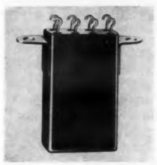
Type JSH relays are spdt and dpdt units with sensitivities of 25 and 40 mw respectively. Non-inductive contact rating is 2 amp at 29 v dc or 1 amp at 115 v ac. The relays can withstand vibration of 15 g from 55 to 2000 cps, 0.09 in. double amplitude from 5 to 55 cps, and shock of 50 g without contact chatter. The units weigh 1.1 oz.
