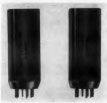
These magnetic-core circuits, including shift registers, pulse gates and core drivers, operate from 0 to 250 kc and are physically and electrically compatible with the T-Series transistor circuits. One core in these circuits will produce the flip-flop action of two transistors. The units are packaged in T-Series containers measuring 7/8 in. in diameter and 2-3/16 in. long, and fit miniature tube sockets.
