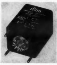
This data-amplifier converter has a high input impedance for use in airborne instrumentation applications requiring the amplification and conversion of millivolt-level ac data signals. Gain stability is  $\pm 1\%$  over the temperature range of -55 to +100 C. Silicon transistors are used. Applications are in strain-gage data systems, servoamplifier systems, and synchro position transmitter systems
