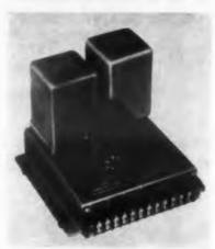
The Series 8000 thermistor temperature control consists of a magnetic amplifier relay, a built-in dc power supply, and two legs of a bridge circuit designed to monitor and control small variations in temperature. When coupled to a thermistor and reference resistor, the bridge can detect temperature variations as small as 0.1 C. Model 8001 will handle 1 amp loads, while Model 8002 will switch up to 5 amp.
