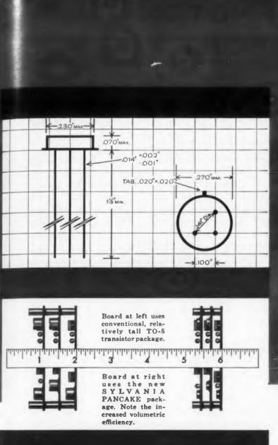
Tentative data MAXIMUM RATINGS AT 25°C SYL-1986 SYL-1987 Collector to Base Voltage 25V -25V Collector Current 100mA 200mA Power Dissipation 100mW 100mW Temperature Range -55°C to +100°C -55°C to +100°C Alpha Cutoff Frequency (min.)\* 4Mc  $*(V_{cb} = 6V, I_e = 1.0mA) (V_{cc} = 6V, I_c = 1.0mA)$
