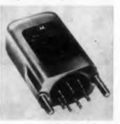
The F5A magnetic modulators have a standard frequency range of 60 cps to 10 kc but can operate as high as 100 kc with low-impedance units. The dual-channel type F5A113 has a signal winding resistance of about 700 ohms. Single-channel type FSA114 is also offered. Originally intended for use as a circuit element in conjunction with amplifiers in servo systems, the units can also be used with thermocouples, strain gages, computing devices, and telemetering equipment.
