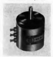
The 2100 Series Micropot, wirewound potentiometers have a 7/8 in. diam and are available in 10-turn and 3-turn models. Resistances to 100 K are offered. The assemblies can withstand over 1 million revolutions without exceeding tolerances. Servo or bushing mountings are available. Zero-based or independent linearity is offered. Units will withstand 1000 v rms between shaft and terminals. MIL specs for environment
