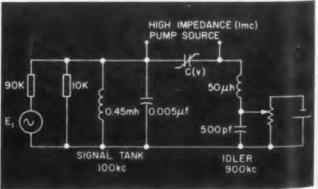
Fig. 1. One-mc parametric amplifier uses the nonlinear reactance of a Zener diode.
