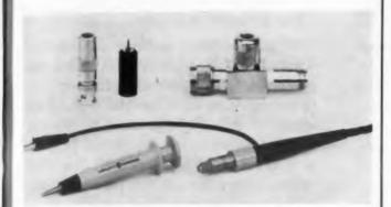
Part of the selection of probes for the 411A RF milli-voltmeter.
