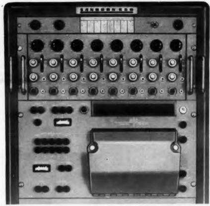
The Sanborn "650" is the first complete multi-channel high-speed optical recording system with medium gain general purpose amplification for each channel. Either the 8-channel amplifier or the recorder may be used separately. Together they provide a max. sensitivity of 2.5 mv/in and a frequency response of DC to 5000 cps (within 3 db at 4 in peak-to-peak) in a multi-channel "direct writing" system.
