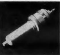
The type D-1008, a ceramic-metal power triode designed to withstand environmental extremes, is a water-cooled tube with a heavy-wall copper anode and mesh-type cathode. The tube is rated at 60 kw, full-power input to 50 mc and reduced input to 110 mc, with maximum anode dissipation of 20 kw. Applications include use as a class C amplifier, or as an oscillator in dielectric and induction heating service. The tube can switch 220 amp at 18 kv as a hard-tube radar modulator.
