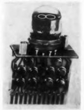
Types TR-40 and TR-57 driver modules are designed to operate the miniature Nixie and the standard and super Nixie indicator tubes, respectively. The driver circuits employ 10 npn transistors in breakdown condition, with current limited by the indicator tube. Signals of 3 v at 300 µa are sufficient to trigger the circuits. The modules are designed for panel mounting and for operating temperatures of -30 to +55 C.
