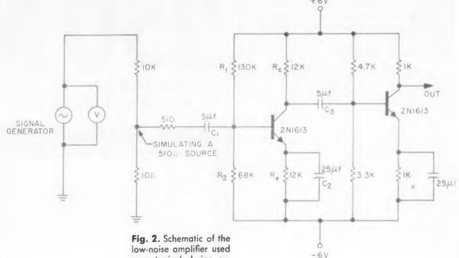
Fig. 2. Schematic of the low-noise amplifier used as a typical design example. The noise level, using unselected 2N1613 transistors, is approximately 18 µv p-p.
