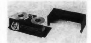
The Type TP-813 tape programer is designed to withstand severe operating conditions encountered in missile, aircraft and ordnance equip-
