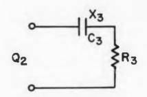
Fig. 2. The parallel  $R_2C_2$  combination of Fig. 1 can be replaced by the series R<sub>3</sub>C<sub>3</sub>.
