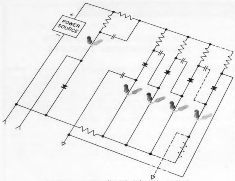
\*SHOCKLEY 4-LAYER DIODES used in typical multiple-stage ring counter circuit.
