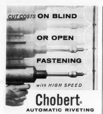
The fastest blind riveting method known...gives uniformly excellent fastening every time. One man, even unskilled, easily completes rivet installation from one side of the work in either open or blind riveting applications in less than 2 seconds. Up to 2000 rivets an hour can be set on production line work.
