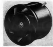
The non-stall blade of this air-mover, Model BC 1607V-1, eliminates the dip in the pressure-flow curve. The unit has a 3-in. over-all diameter and is 2-5/16 in. long. It weighs 15 oz and is designed for 115 v, 400 cps, although units with other power requirements are available. The air-mover, suitable for cooling compact components in missiles, submarines and aircraft, meets MIL specs for environment and performance.
