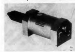
The Series P2-1253 pressure transducers are applicable where interest lies primarily in the upper end of a pressure transducer's range, that is from 475 to 550 psi. Full 0 to 5 v de output is concentrated in this portion of the range, rather than being dissipated in areas of no interest. Units have high output with no amplification needed. Accuracy is better than 0.15%.
