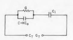
Fig. 3. Equivalent circuit of an entire probe system.
