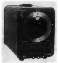
Model 401-B oscillator, a source of audio and ultrasonic sine waves, operates with a distortion of less than 0.1% at full output of 20 v, open-circuit. Frequency range is 9 cps to 120 ke, covered in four decade bands. Accuracy is  $\pm 2\%$ . Output amplitude is controlled by a five-position decade attenuator plus a continuous control; any voltage above 100 mv can be selected. Output amplitude is independent of frequency within  $\pm 0.5$  db. The unit measures 8 x 6 x 10.5 in. and weighs 12 lb.
