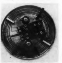
These wire sonic delay lines use piezoelectric transducers for the inputs and fixed outputs and magnetostrictive transducers for the adjustable outputs. Available delays are 2 µsec to 20 msec, with  $\pm 0.1$  µsec tolerance. Maximum operating frequency is 1.25 mc. Piezoelectric drives have a power loss of 10 to 15 db; magnetostrictive types have losses of 20 to 25 db. Output amplitude is stable, generally within 10% for changes in input frequency, repetition rate or temperature.
