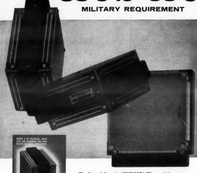
The General Ceramics MICROSTACK, one of the most important advances in memory core packaging, now operates in a temperature range of from —55°C to +85°C. Core characteristics remain constant. By maintaining temperature stability inside the MICROSTACK unit, General Ceramics engineers have developed a memory core package that is smaller, more rugged, requires no external cooling or heating, and meets MIL shock and vibration specifications.
