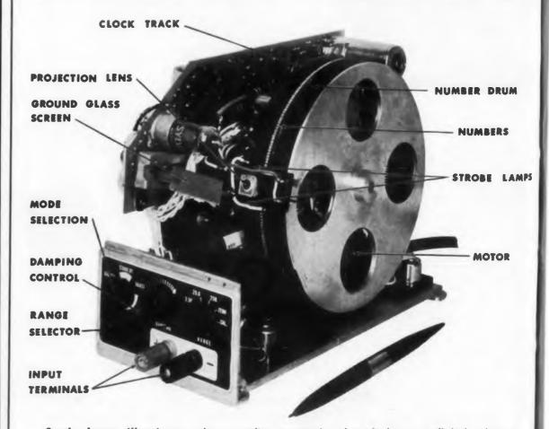
Strobe lamps illuminate voltage reading on rotating drum in low-cost digital voltmeter.
