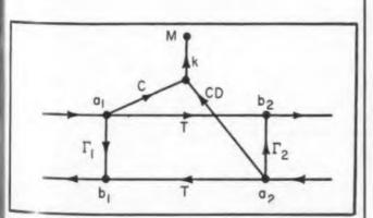
Fig 3b. With only two available rf ports, network flow raph can be simplified.
