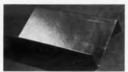
Heated dies are not necessary with Special Bend sheet.
