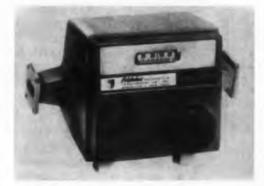
Type 101 broadband, direct-reading attenuators come in nine models covering the frequency range of 3.95 to 40 kmc. Attenuation range is 60 db and maximum vswr is 1.15. The units are rotary-vane type. The value of attenuation is deemined by the angular position of a resistive film with respect to the wavegiude.
