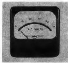
are accurate to 1%. Parts are machine turned, with spring-mounted jewel bearings. Meter ranges are from 50 µa to 500 amp dc, 100 µa to 20 amp ac, 10 mv to 750 v de, 8 to 500 v ac. Ac meters are rectifier type. Meters measure from 2-1/2 to 6-3/4 in. sq.
