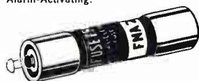
FNA FUSETRON Fuse 13/32 x 1/2 in. slow-blowing, Visual-Indicating, Alarm-Activating. (Also useful for protection of small motors, solenoids, transformers in machine tool industry.)
