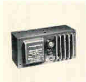
Modular power supplies series AN3000 measure 2\frac{3}{4} \times 6 \times 3\frac{1}{8} in. over-all, and provide all voltages necessary for the operation of practically any combined analog-digital, discrete, hybrid, or integrated circuitry. All four models in the series use silicon semiconductors and operate from 0° to 70°C. Prices, $94.50 to $124.50. Analogic Co., Newton St., Waltham, Mass. [385]
