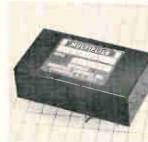
Plug-in analog multiplier model AM701 combines solid state integrated circuitry with the proven magnetoresistor bridge to obtain analog multiplication. It accepts \pm 10 -v signals and delivers \pm 10 -v output at 5 ma with a one quadrant accuracy of \pm 0.40\% of full scale. Price in lots of 1 to 24 is $98.50 each. American Aerospace Controls Inc., Farmingdale, N.Y. [387]
