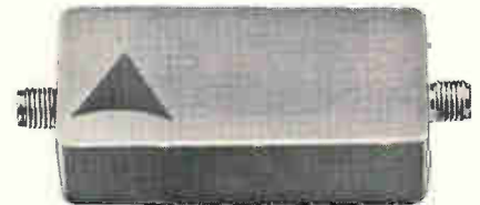
Slowdown. A piezoelectric film at the input converts an electrical signal into a slower-moving acoustic one.
