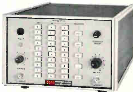
MODEL 4100 SOLID STATE PUSH-BUTTON VARIABLE OSCILLATOR covers 0.01 Hz to 1 MHz, with simultaneous sine- and square-wave outputs. Size: 8½"W x 5¼"H x 14½"D. Price: $550.
