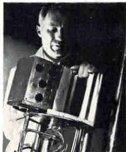
Target ready. A technician positions the target. On his right is the five-sided substrate holder
