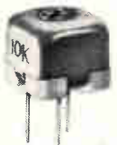
Series 340 Top Adjust 1/4" x 1/4" x .220" Cermet Trimmer
