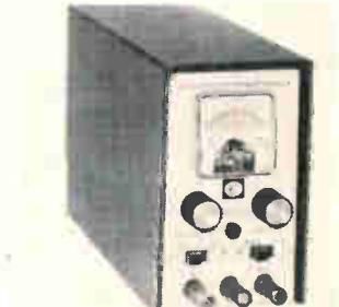
Regulated d-c power supplies are available in two models: PSR-12-25 with output from 0 to 25 v d-c, 0 to 500 ma, and PSR-12-50 with output of 0 to 50 v d-c, 0 to 250 ma from input of 105 to 125 v 60 hz. Line regulation is 0.01% +2 mv, load regulation is 0.01%. Ripple is less than 100 microvolts. Electro Products Laboratories Inc., 6125 Howard, Chicago. [388]
