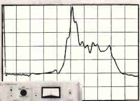
Autocorrelation of bat cry defined by Model 100 Correlation Function Computer (Price: $8,500.)
