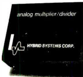
Analog multipliers models 103 and 104 offer full scale accuracy better than 0.1% for full 4 quadrant operation. The transfer function of the 103 is +XY/10, whereas the 104 is -XY/10. Both units may be used to multiply, divide, square, and square root by appropriate pin interconnections. Price (1-9) is $325. Hybrid Systems Corp., 95 Terrace Hall Ave., Burlington, Mass. [386]
