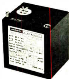
Static inverter model N2D converts 28 v d-c to 400 hz sine wave voltages of either 115 or 26 v a-c. With continuous full load operation at 160° F, it supplies an output power of 20 v-a. Modular design provides a package as small as 2½ x 3 x 3¼ in. which weighs less than 2.1 lbs. Price is $218. Abbott Transistor Laboratories Inc., 5200 W. Jefferson Blvd., Los Angeles 90016 [381]
