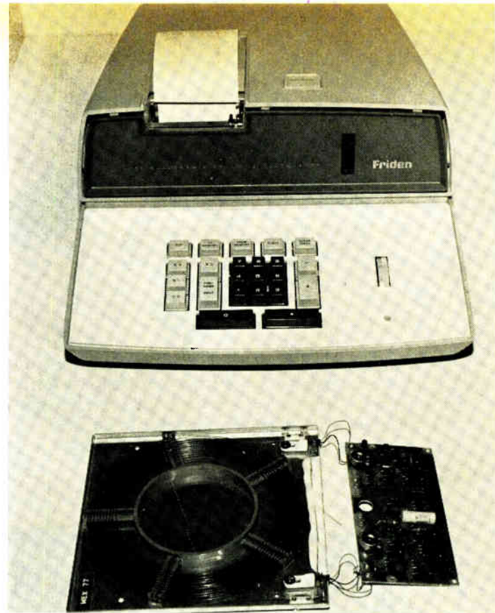
Line of action. The 1150 printing calculator's operation depends on the delay line in the foreground.
