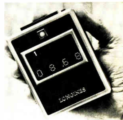
Good timing. Light-emitting diodes produce readout in stop watch.
