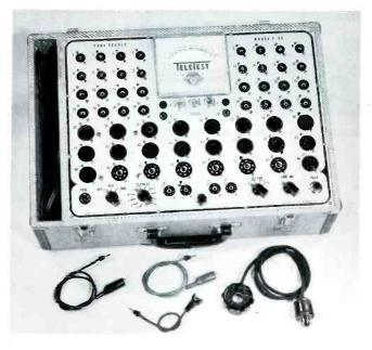
Fig. 4. Another Tube Checker for Rapid Testing.
