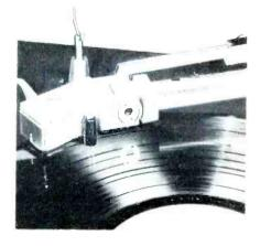
Fig. 4. Eby Stati-Mute Installed on General Electric "Baton" Arm.
