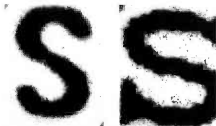
A CHARACTER GENERATED BY THE TFEL EDGE EMITTER (left), is clearer than that from a laser-light source (right). Both images are magnified 50 times.
