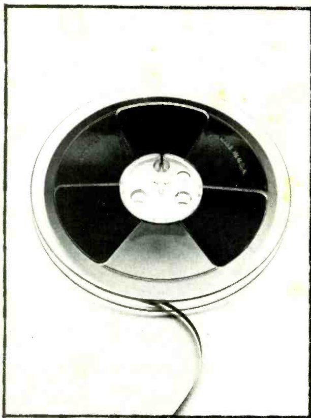
Open-reel tape is wound in a pancake shape on a plastic reel similar to home movie-film reel.
