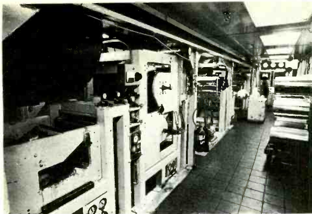
Above is but a small part of one of the giant coating machines: in this section the film is fed into the machine, coated, and exposed to a magnetic field to orient the iron-oxide particles.
