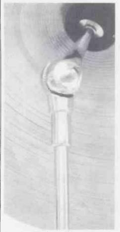
The tilter on the cymbal stands is the screwdriver-type, but the lugs on the drums are the square type, so the keys won't fit.
