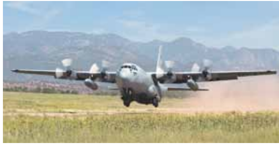
A C-130 aircraft from the Air Force Reserve Command's 302nd Airlift Wing prepares to land on an unimproved runway during training at Red Devil tactical airstrip at Fort Carson, Colo. These landings cause rocks and other debris to hit the underside of the aircraft. The 302nd Maintenance Group started adding protective tape to the struts to alleviate the damage. (U.S. Air Force photo/Chief Master Sgt. James Riley)
