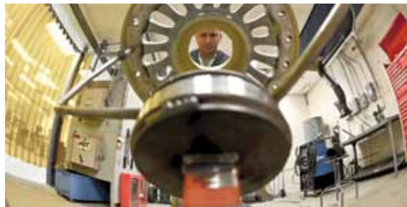
Staff Sgt. Alex Aguayo 6th Maintenance Squadron aircraft metals technician inspects a newly fabricated wheel workstation, Aug 20, 2013 at MacDill Air Force Base, Fla. Aguayo co-engineered a stand to hold the wheel, which reduces the man hours needed to paint by 26 man-hours per set. (U.S. Air Force photo/Staff Sgt. Brandon Shapiro)
