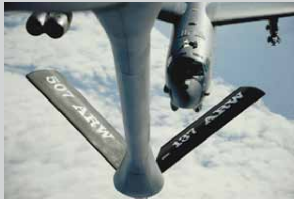
A B-52 Stratofortress prepares for a fuel delivery from a KC-135 Stratotanker in support of exercise Rim of the Pacific exercise, or RIMPAC July 10, 2010, over the Pacific Ocean. (U.S. Air Force photo/Staff Sgt. Kamaile O. Long)
