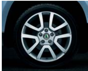
Spitzberg 7.0J x 17" alloy wheels for 225/50 R17 tyres are standard on the 103TDI 4x4 model.
