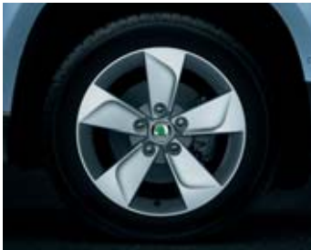
Nevis 7.0J x 16" alloy wheels for 215/60 R16 tyres are standard on the 77TSI model.
