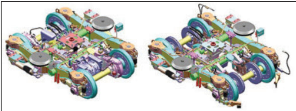
Figure 8.4 CRH380A Motor Bogie (left) and Trailer Bogie (right)
