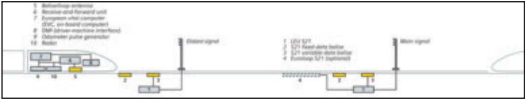
Figure 9.5 Trainguard 100 for ETCS Level 1
