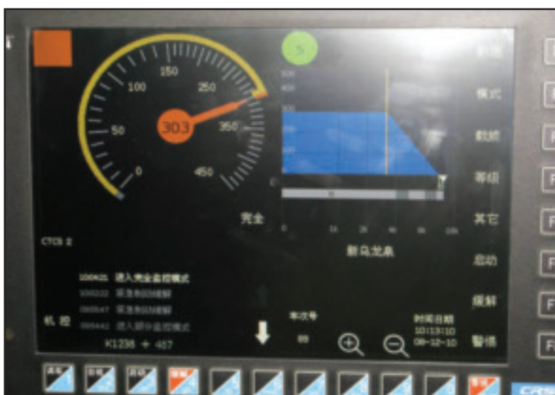
Figure 9.9 CTCS-3 Driver-Machine Interface
