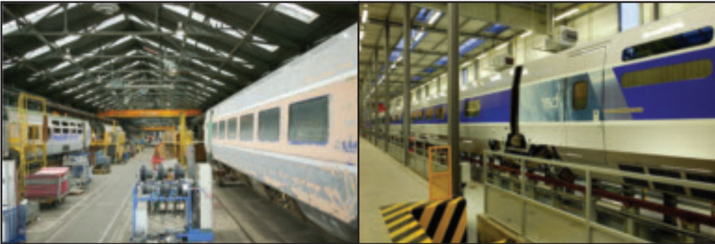
Figure 19.6 TGV Undergoing Major Refurbishment is Prepped for Paint (left) and Newly Painted (right)
