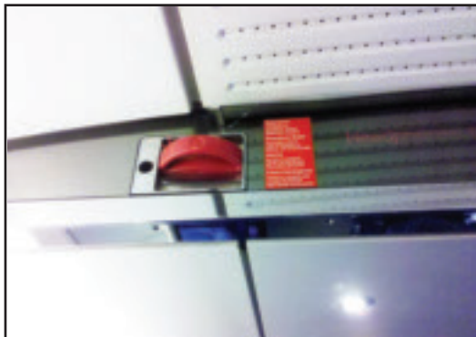
Figure 7.3 Passenger Emergency Brake Device on ICE 3
