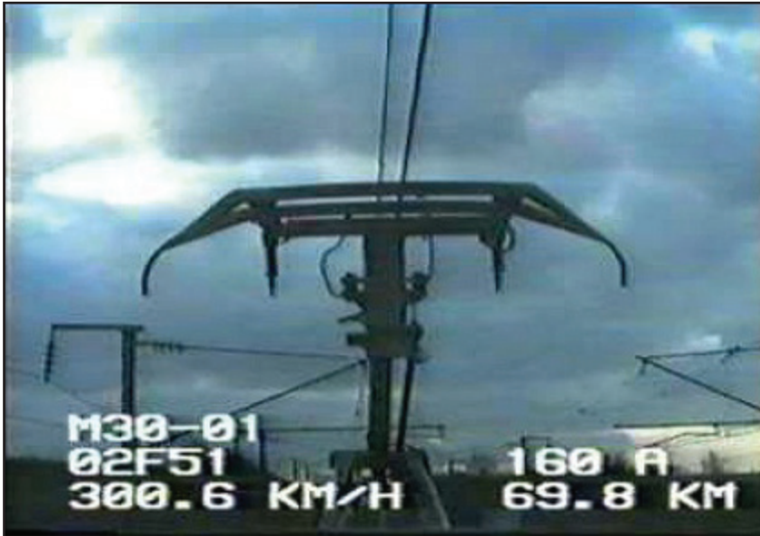
Figure 16.3 Monitoring of Pantograph and OCS Interaction
