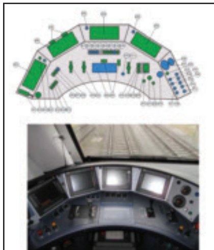
Figure 9.11 UIC 612 Generic Layout of Driver's Desk and Actual Desk on Alstom PRIMA II Locomotive
