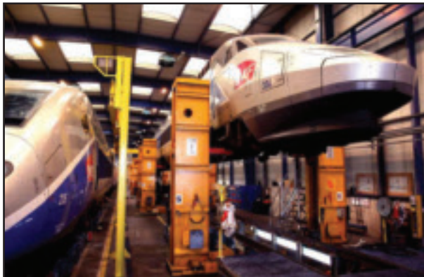
Figure 19.3 Trainset Lift Arrangement at SNCF Technicentre
