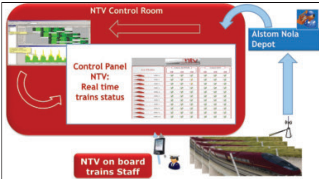
Figure 19.7 Real-Time Monitoring of AGV Trainset Status
