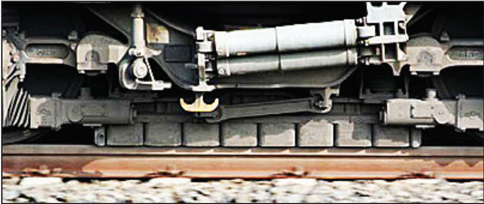
Figure 7.2 Eddy Current Track Brake System on a Siemens ICE 3 Trainset
