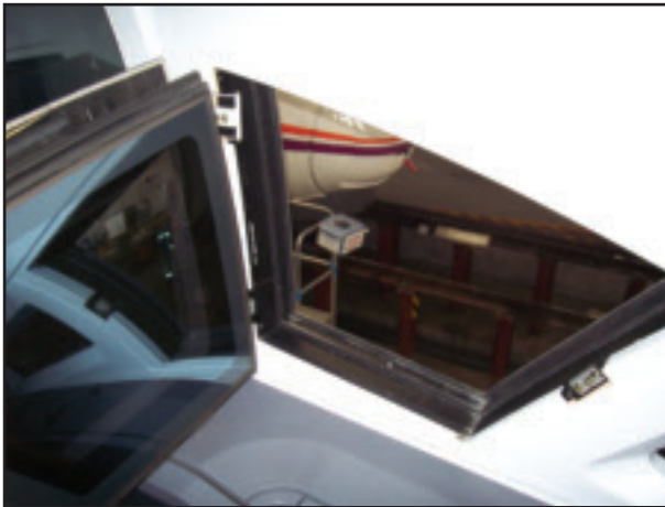
Figure 4.5 Velaro E Cab Emergency Hatch
