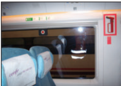
Figure 4.4 Velaro E Emergency Side Glazing with Breakout Hammer
