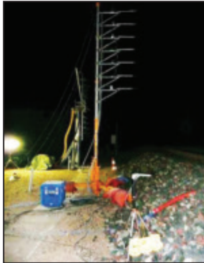
Figure 5.4 Setup for Air Pressure Tests
