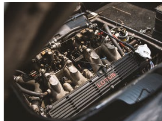
Right: 141PS 2-litre four is unchanged from the standard Esprit of the day. Below: five-speed manual 'box needs decisive action from the driver
