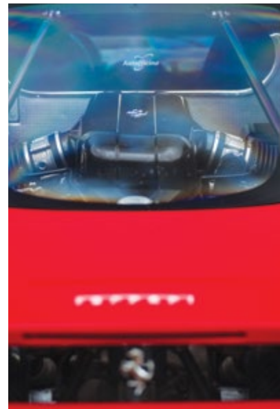
Top: carbonfibre body helped keep the Enzo's weight down to 1255kg (dry). Below right: V12 produces 660PS – still a mighty figure, but down 303PS on the LaFerrari
