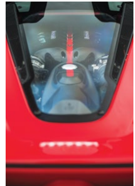
Top: LaFerrari is same length as the Enzo, with an identical wheelbase, but is 43mm narrower; it weighs the same too, despite its V12 (below) being joined by a hybrid system
