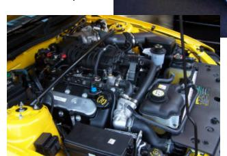
Shelby Mustang Cobra engine with supercharger
