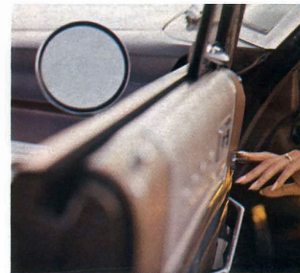
REMOTE-CONTROL OUTSIDE MIRROR With control lever located on inside door panel, driver can conveniently adjust mirror for best vision.
