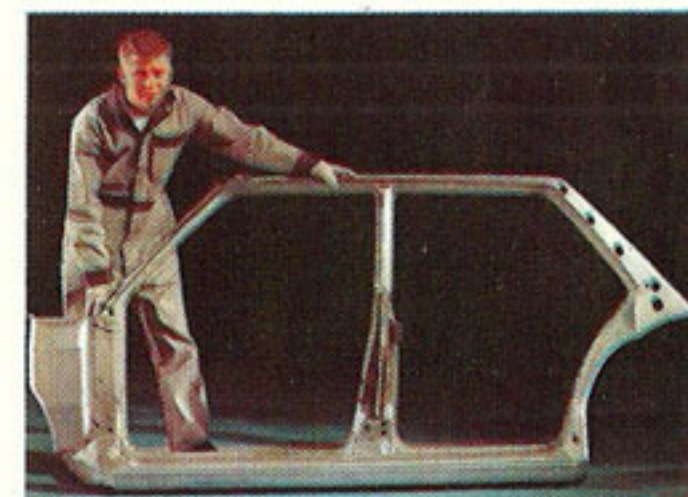
Rambler's Advanced Unit Construction uses exclusive, one-piece uniside. Extra strong.
