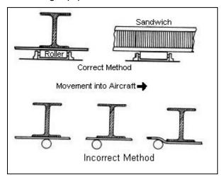
FIGURE 4. Pallet/roller interface.
