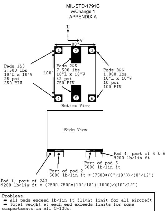
FIGURE A-20. Floor loading calculation.
