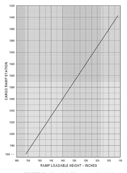
FIGURE B-58. Allowable in-flight ramp loadable height.
