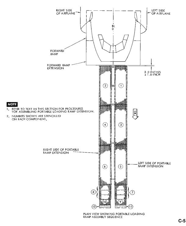
FIGURE B-31. Portable loading ramp extension assembly sequence.
