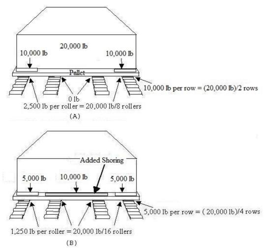
FIGURE A-16. Pallet/roller weight distribution.
