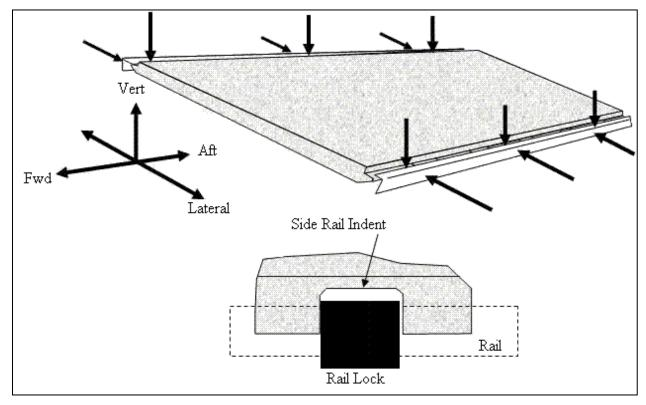
FIGURE A-13. Pallet locked into aircraft rails.
