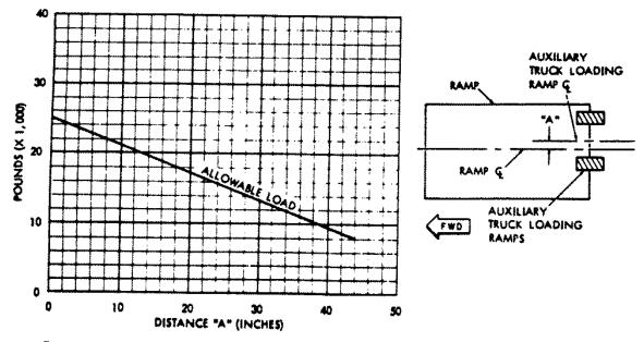
To determine distance "A", measure from the ramp centerline to a point midway between the installed ramps. Find distance "A" on the horizontal scale. Extend a line vertically from this point to the allowable load line. Extend a line horizontally until it intersects the vertical scale. Read the allowable load.
