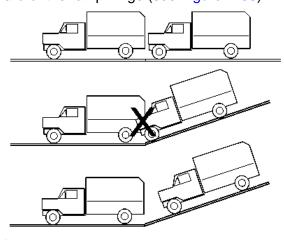
FIGURE A-55. Ramp cargo placement.
