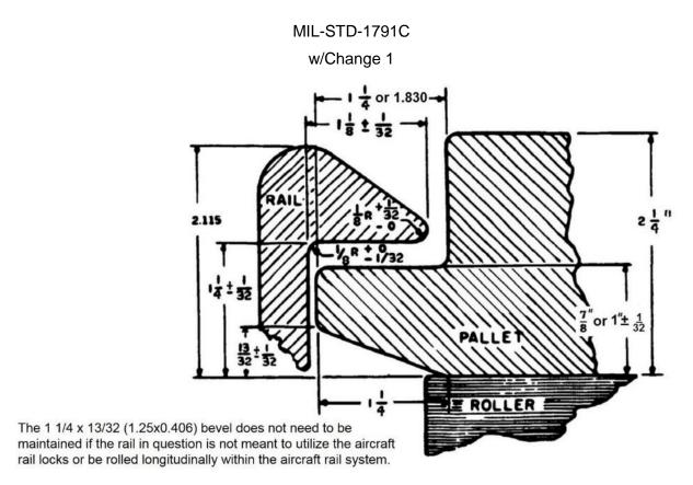
FIGURE 5. Pallet rail exterior profile.
