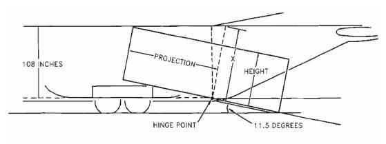
TO CALCULATE THE MAXIMUM CARGO PROJECTION INTO THE AIRPLANE, USE CHART A. EXTEND A LINE TO THE LEFT SCALE FROM A POINT ON THE CHART CURVE DIRECTLY ABOVE THE CARGO HEIGHT ON THE BOTTOM SCALE. READ THE ALLOWABLE PROJECTION. EXAMPLE: CARGO HEIGHT IS 90 INCHES. MAXIMUM PROJECTION IS 99 INCHES.
