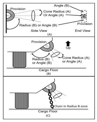
FIGURE A-33. Multiple chain restraint.
