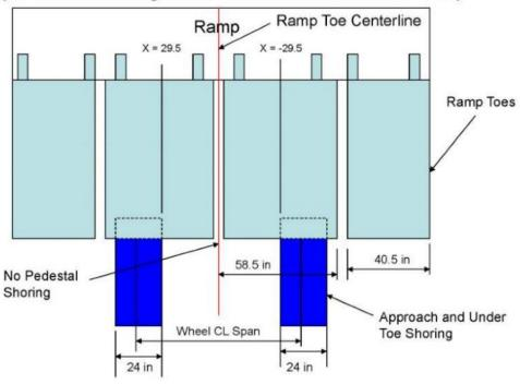
FIGURE B-59. C-17 minimum approach shoring width under ramp toes - (sheet 2 of 4).
