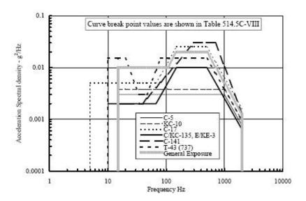
FIGURE 514.5C-6. Jet aircraft cargo vibration exposure.
