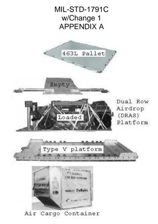
FIGURE A-17. Standard pallets and containers.
