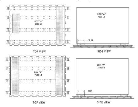
FIGURE A-15. Non-uniform pallet loading.
