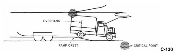
FIGURE B-85. Overhang and projection limits (vehicle).
