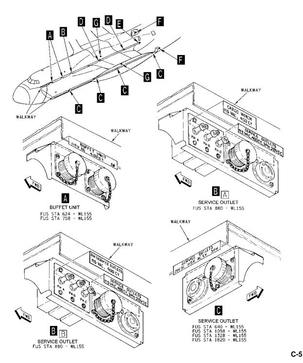
FIGURE B-46. Cargo compartment electrical outlets.
