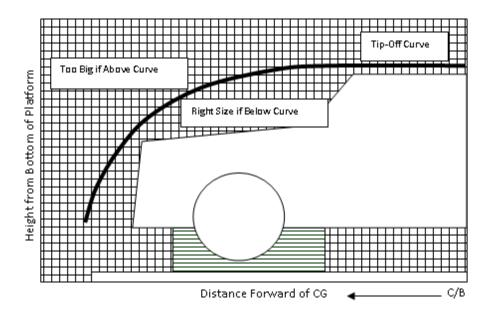
FIGURE A-56. Tip-off curve.
