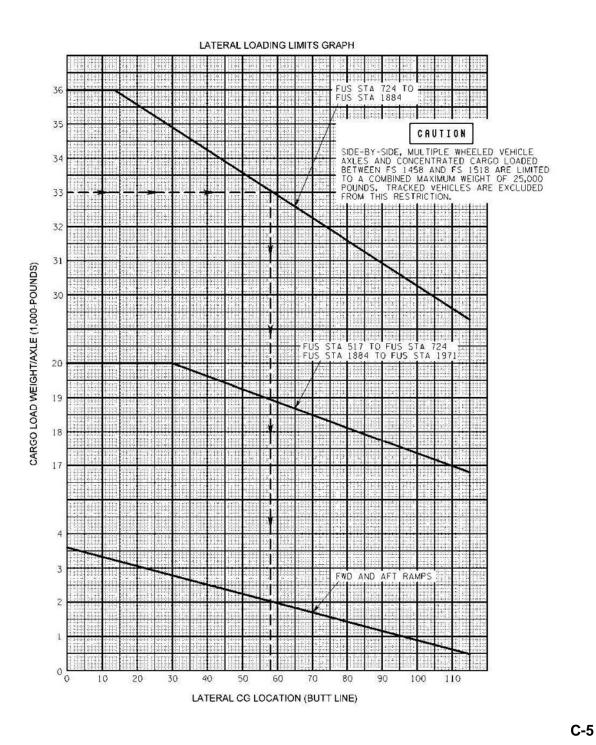
FIGURE B-33. Cargo maximum allowable lateral CG location (sheet 3 of 3).
