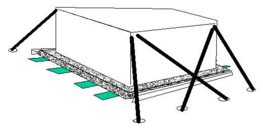
FIGURE A-10. Palletized cargo restrained to aircraft floor rings.
