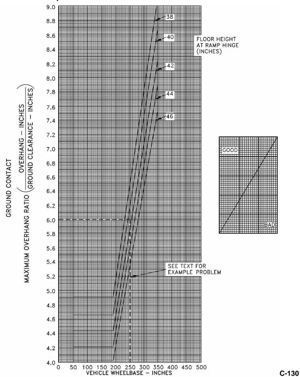
FIGURE B-87. Overhang and projection limits (vehicle).
