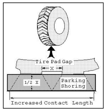
FIGURE A-44. Shoring for large gapped tires.
