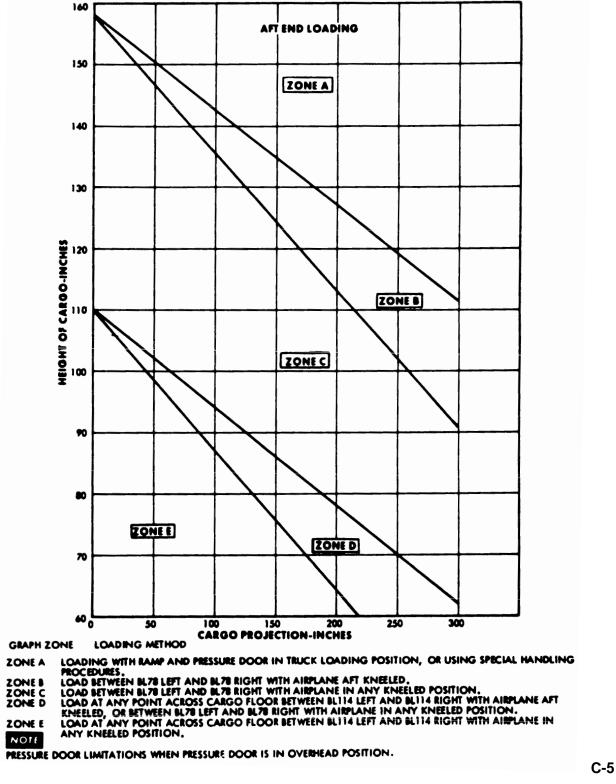
FIGURE B-7. Crated cargo projection limits (forward and aft end loading palletized) - Continued.
