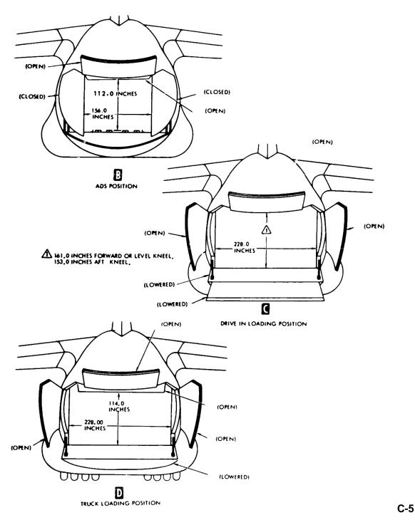
FIGURE B-4. Aft cargo opening dimensions.
