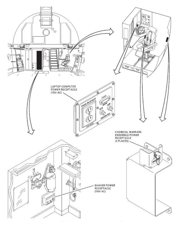
FIGURE B-76. Cargo compartment electrical receptacles.
