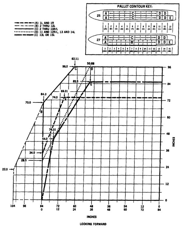
FIGURE B-106. Pallet contours and aisle configurations.
