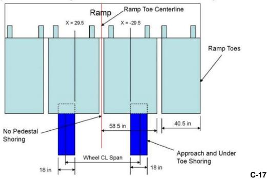
FIGURE B-59. C-17 minimum approach shoring width under ramp toes (sheet 1 of 4).
