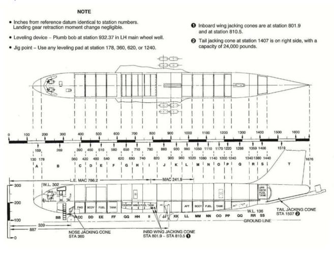
FIGURE B-126. Aircraft diagram (typical).
