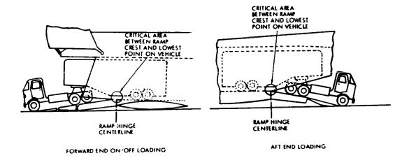
FIGURE B-22. Forward and aft ramp crest limits.
