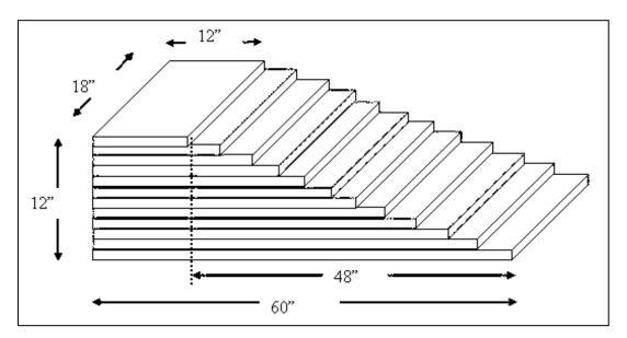
FIGURE A-38. Sample approach shoring stack.
