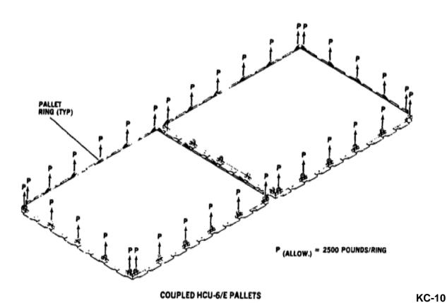
FIGURE B-121. HCU-6/E pallet ring vertical allowables.
