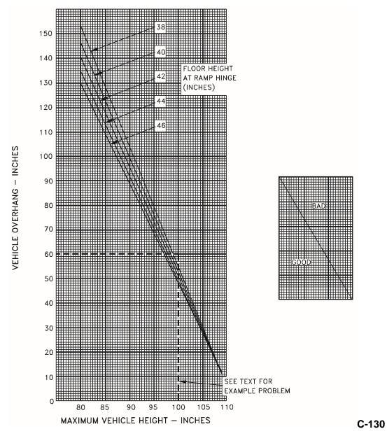
FIGURE B-85. Overhang and projection limits (vehicle) - Continued.
