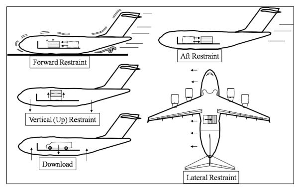
FIGURE A-22. Restraint for various situations.
