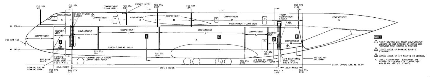
FIGURE B-6. Airplane kneeling loading position (on/off loading).
