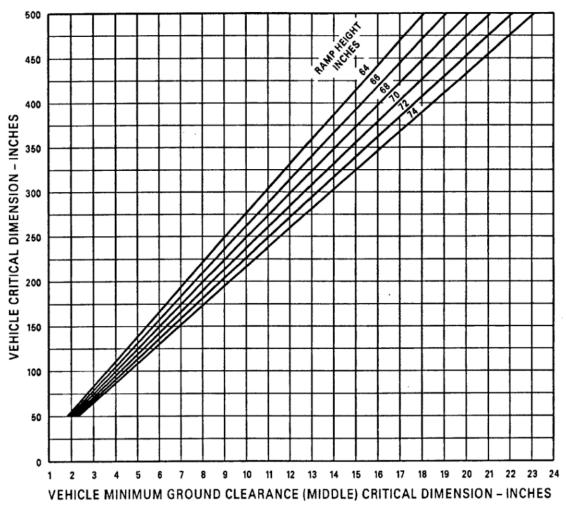
FIGURE B-56. Vehicle ramp crest clearance limit.
