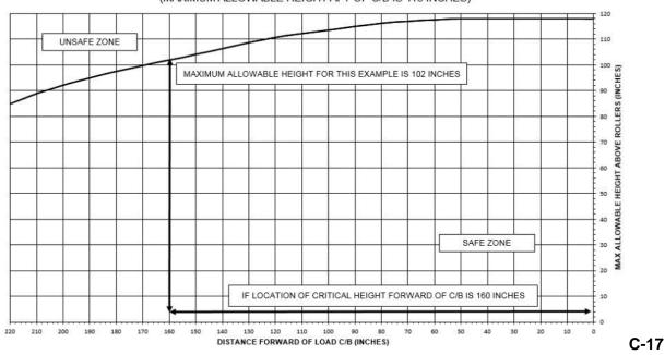
FIGURE B-77. C-17 tip off curve.
