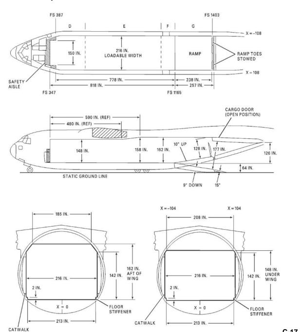
FIGURE B-48. Cargo compartment loading envelope.
