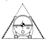
FIGURE A-30. CG location for effective restraint.
