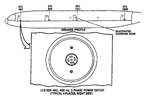
FIGURE B-123. Cargo compartment electrical outlets.
