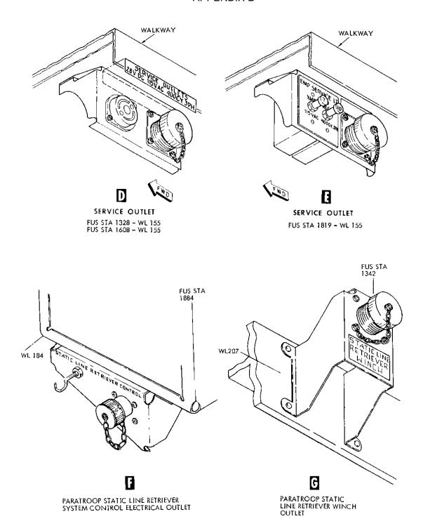
FIGURE B-46. Cargo compartment electrical outlets - Continued.
