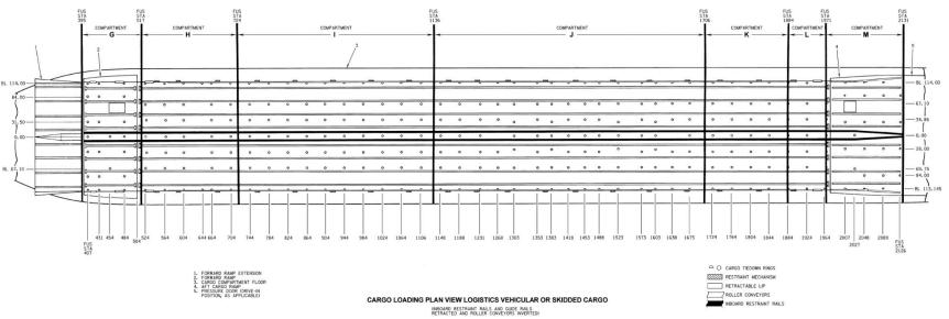
FIGURE B-43. Cargo floor configuration (ADS cargo).
