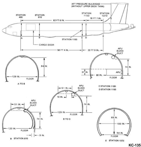
FIGURE B-127. KC-135 R/T cargo compartment.
