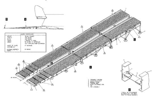
FIGURE B-30. Portable loading ramp extension.
