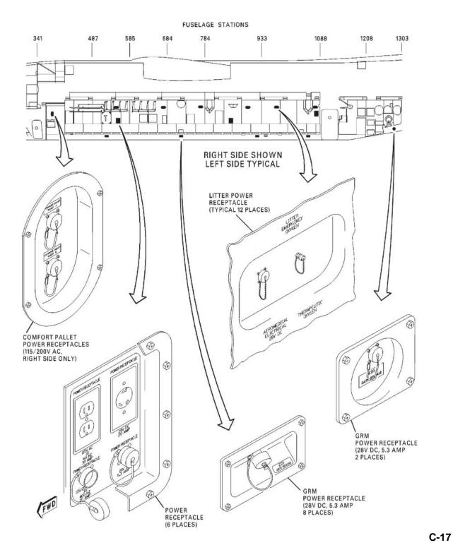
FIGURE B-76. Cargo compartment electrical receptacle - Continued.
