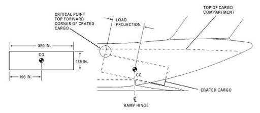
FIGURE A-19. Projection of bulk cargo.
