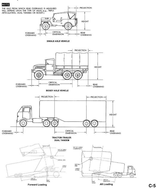
FIGURE B-7. Crated cargo projection limits (forward and aft end loading-palletized).
