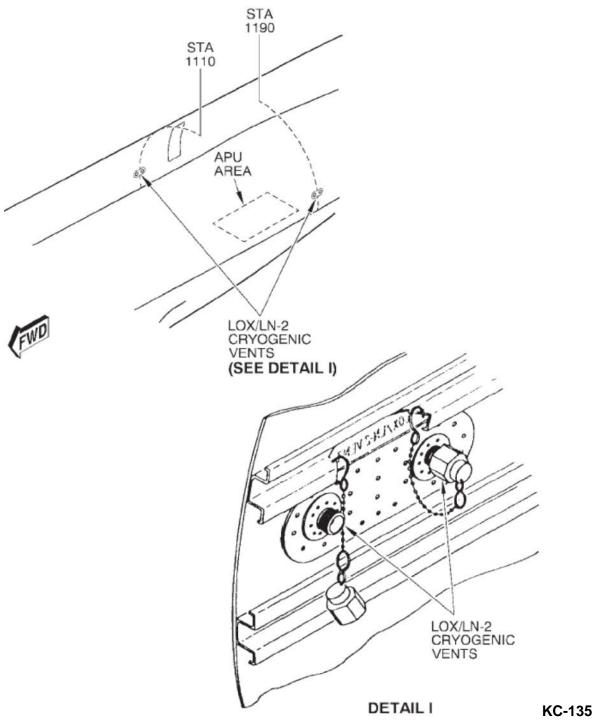
FIGURE B-137. KC-135 cryogenic vents.
