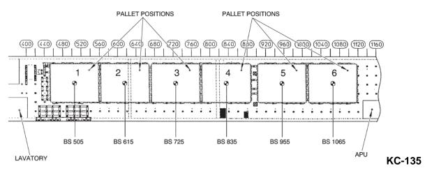
FIGURE B-128. Cargo roller handling system (six pallets installed).
