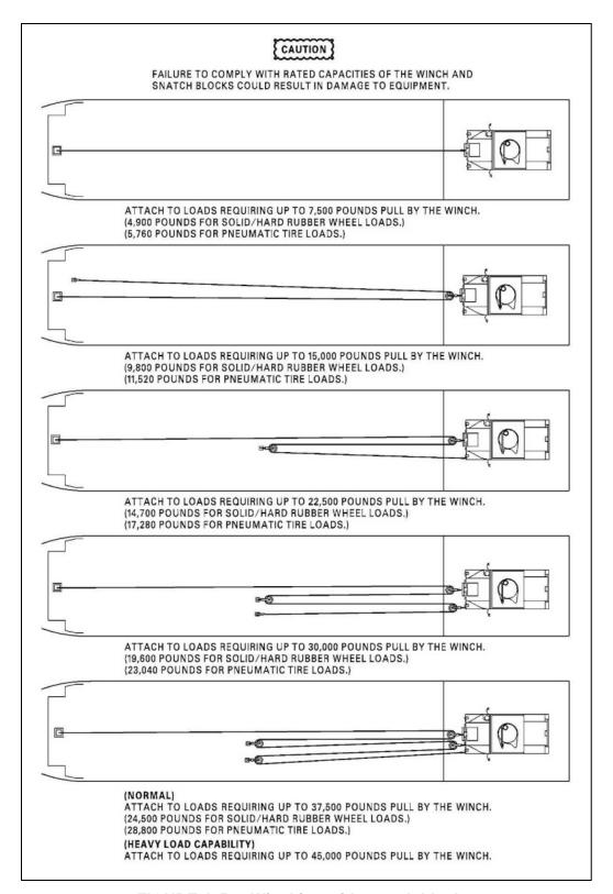
FIGURE A-50. Winching with snatch blocks.
