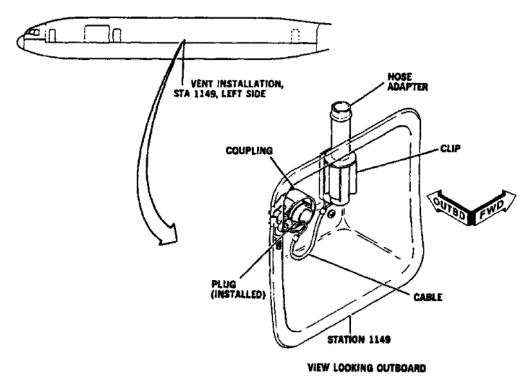
FIGURE B-122. Cargo compartment cryogenic vent.
