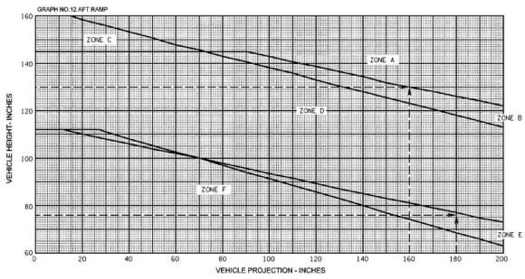
FIGURE B-21. Forward and aft end loading vehicle projection limits.
