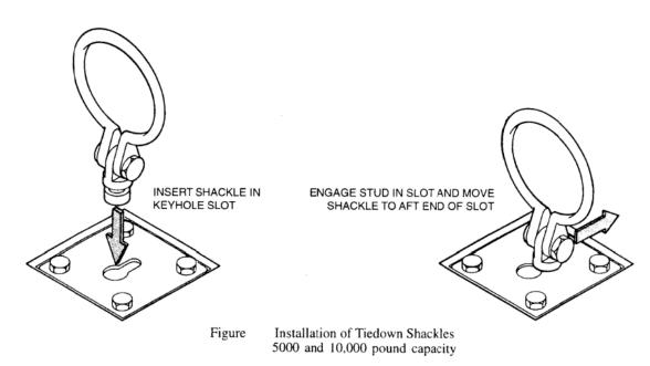
FIGURE B-135. Installation of tiedown shackles 5,000 and 10,000 pound capacity.
