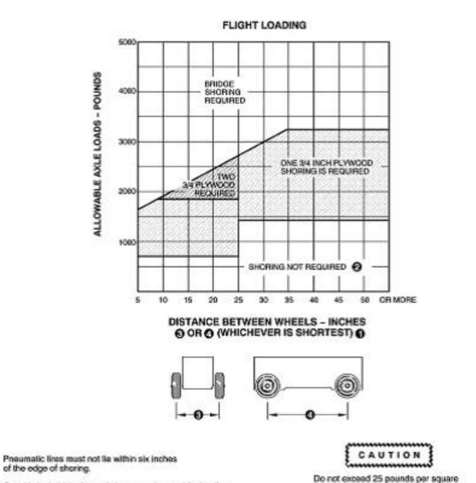
FIGURE B-132. Allowable axle loads for pneumatic tires - Continued.
