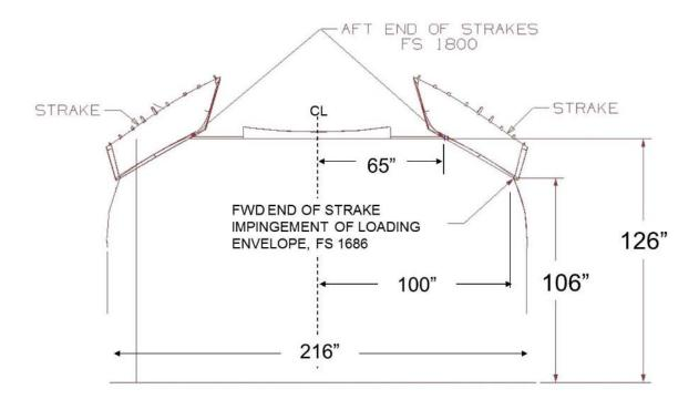
FIGURE B-50. C-17 straight-in loading envelope, end view.
