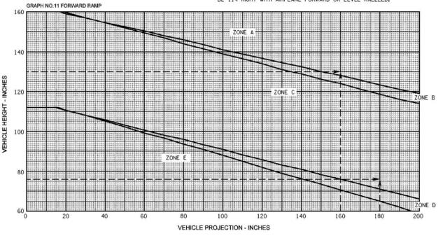
FIGURE B-20. Forward and aft end loading - vehicle projection limits.
