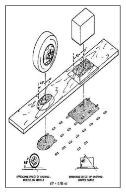
FIGURE A-42. Shoring to spread weight.
