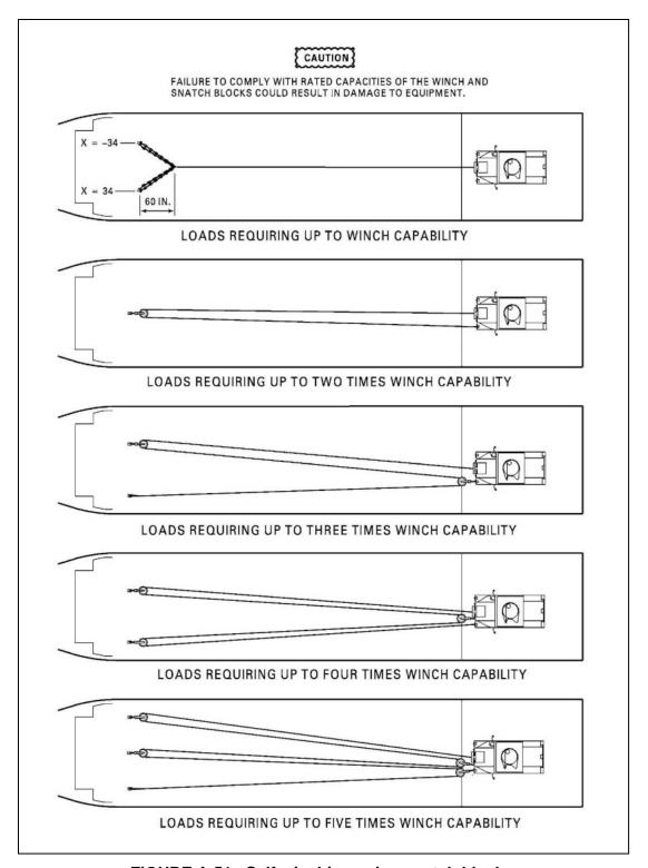
FIGURE A-51. Self-winching using snatch blocks.
