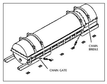
FIGURE A-29. Chain gate and chain bridle.
