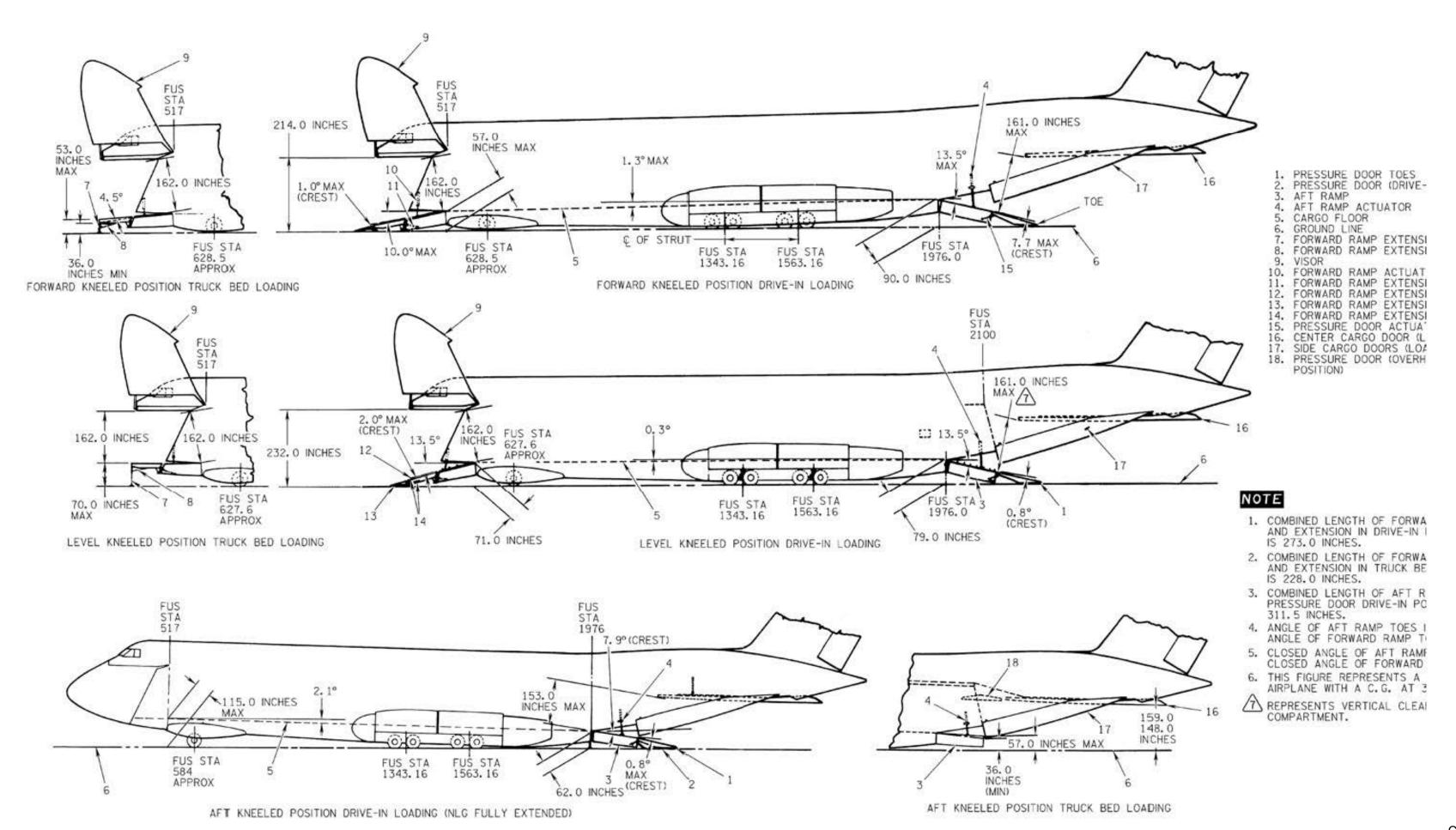
FIGURE B-6. Airplane kneeling loading position (on/off loading) - Continued.
