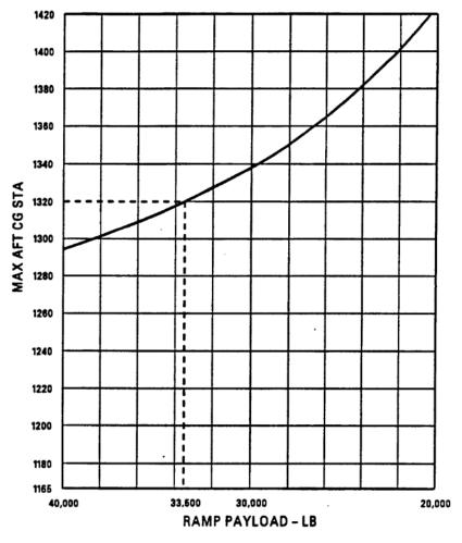
FIGURE B-70. Allowable in-flight ramp payload.
